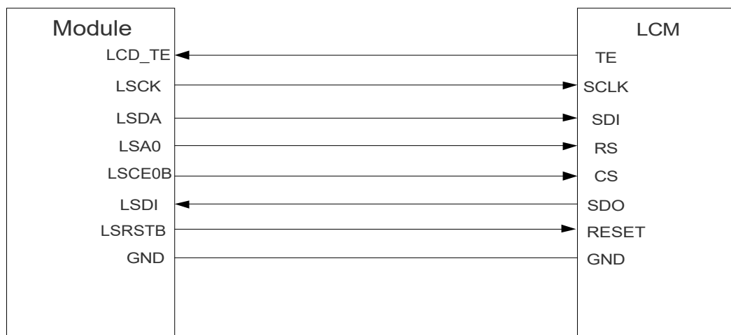
Figure 25: Reference Circuit Design for LCM Interface
