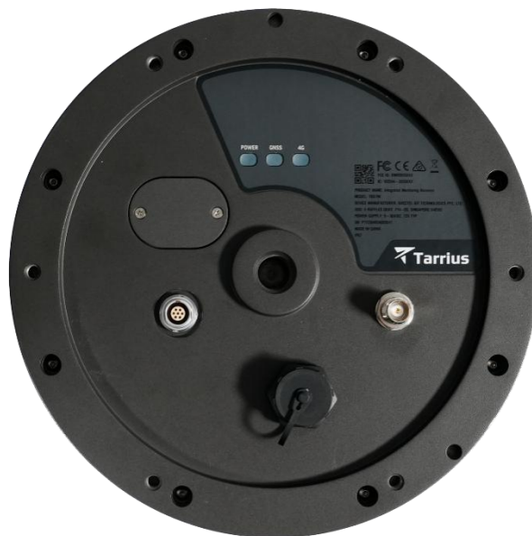
Figure 2: TR07M Integrated Monitoring Receiver (Bottom View)
