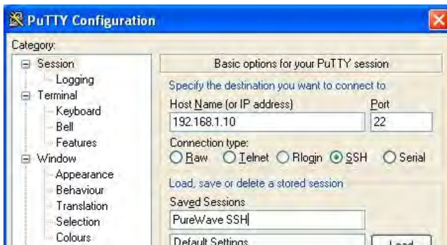
Figure 7 PuTTY SSH Client Configuration
