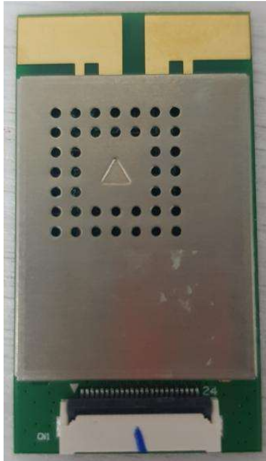
Fig 7.1 Pin sequence of 5G_MODULE_FPC Module
