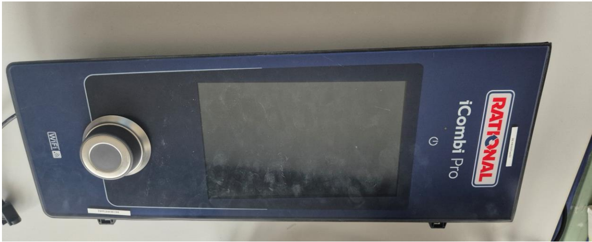
Figure 1: WA112 PCBA housing TOP side example (including Display, Capacitive touch and PushTurn-Key. Note: This housing is provided by RATIONAL AG.
