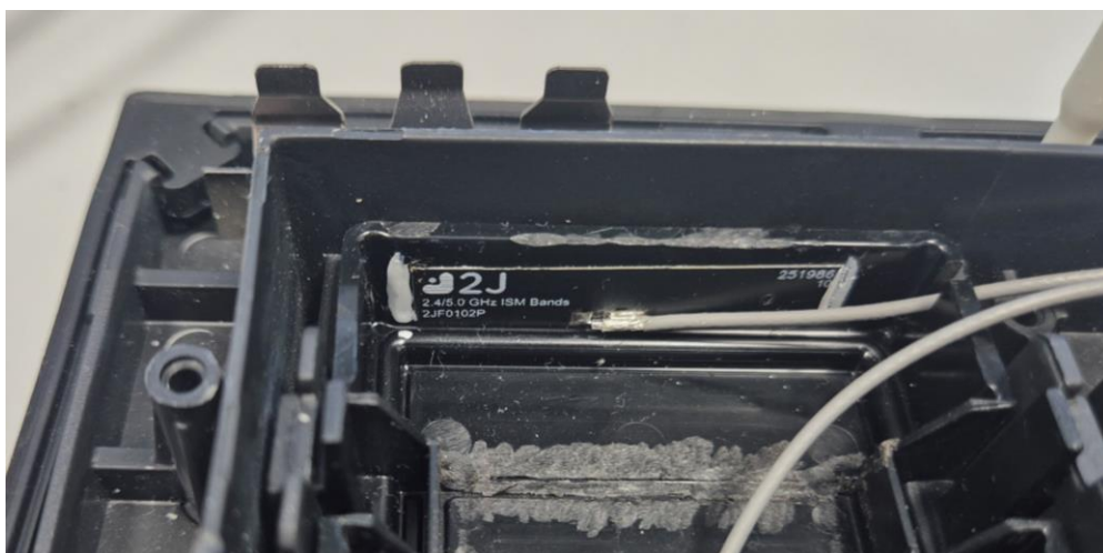
Figure 4: WA112 PCBA housing BACK side example (including Display, Capacitive touch and PushTurn-Key. Note: This housing is provided by RATIONAL AG. WA112 PCBA is mounted. Detail view of WIFI antenna placement
