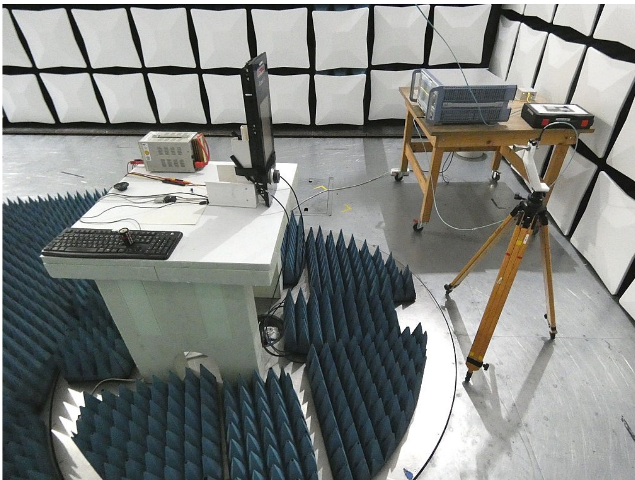
Photo 16: Test setup for radiated measurements (AC Port (power line), EUT supplied by laboratory power supply, 26 to 30 GHz, unintentional radiator §15.109, ANSI C63.4), view from right side
