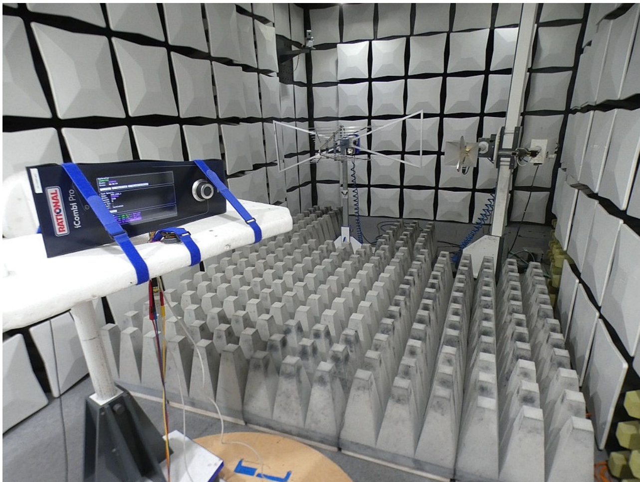
Photo 1: Test setup for radiated measurements (Enclosure, fully-anechoic chamber, 1-26 GHz intentional radiator §15, ANSI C63.10 and §22/24/27/90, ANSI C63.26). EUT on turnunit
