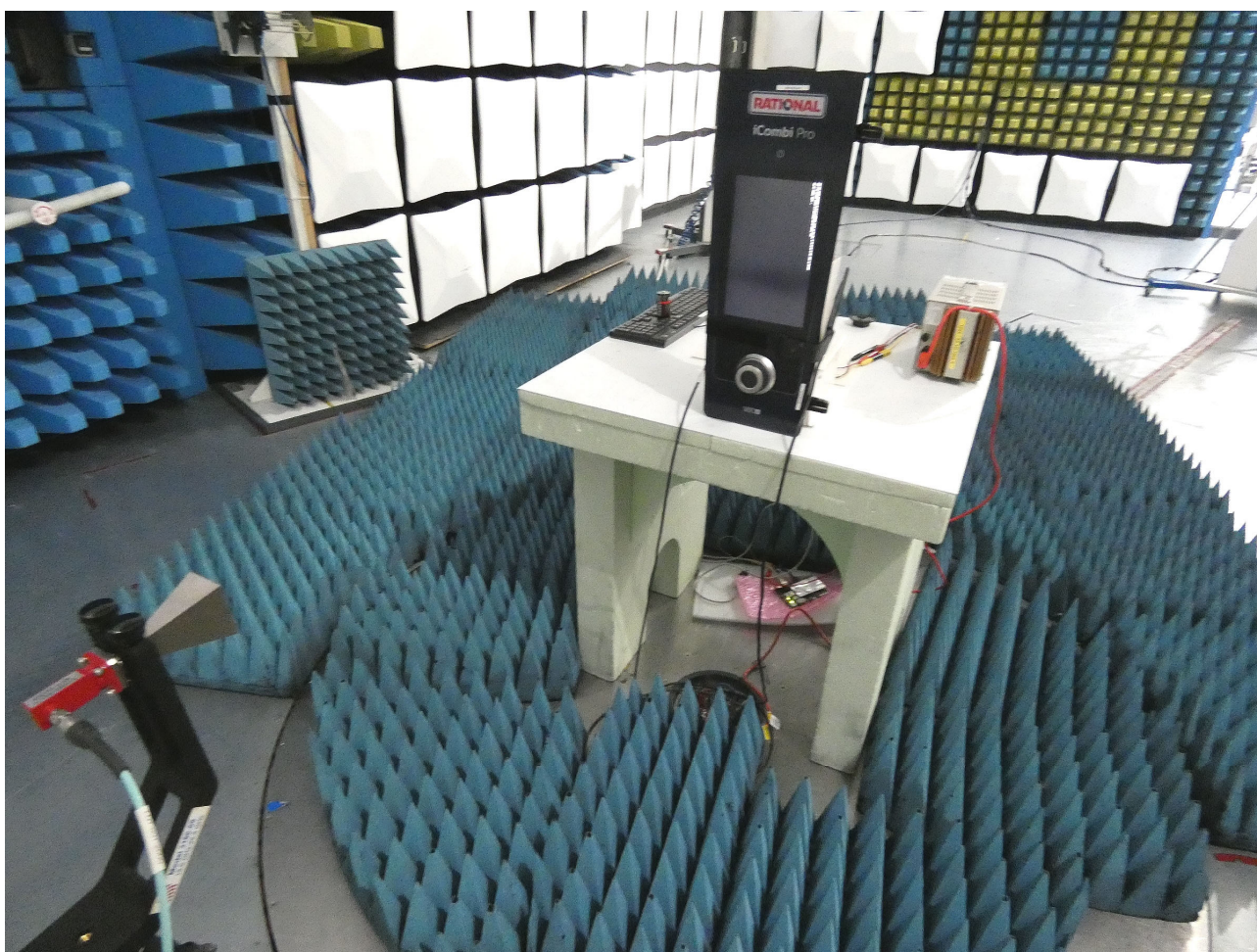
Photo 14: Test setup for radiated measurements (AC Port (power line), EUT supplied by laboratory power supply, 18 to 26 GHz, unintentional radiator §15.109, ANSI C63.4), EUT front view
