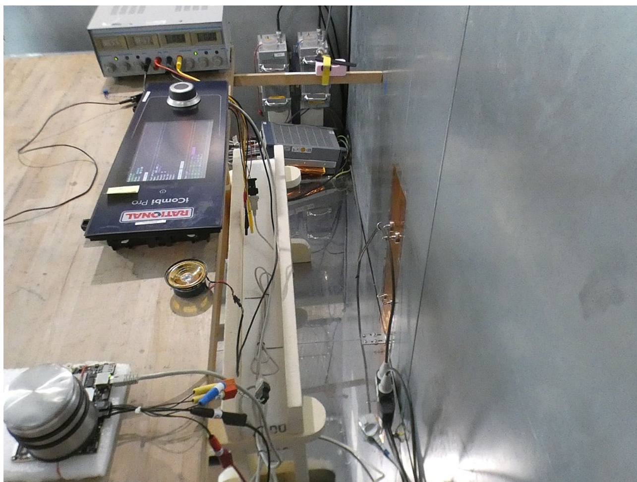
Photo 5: Test setup for conducted measurements (AC Port (power line), EUT supplied by auxiliary laboratory power supply, unintentional radiator §15, ANSI C63.4), rear side
