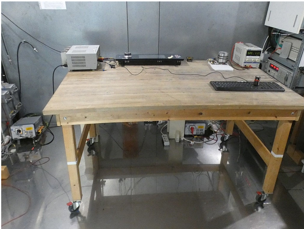
Photo 3: Test setup for conducted measurements (AC Port (power line), EUT supplied by auxiliary laboratory power supply, unintentional radiator §15, ANSI C63.4)
