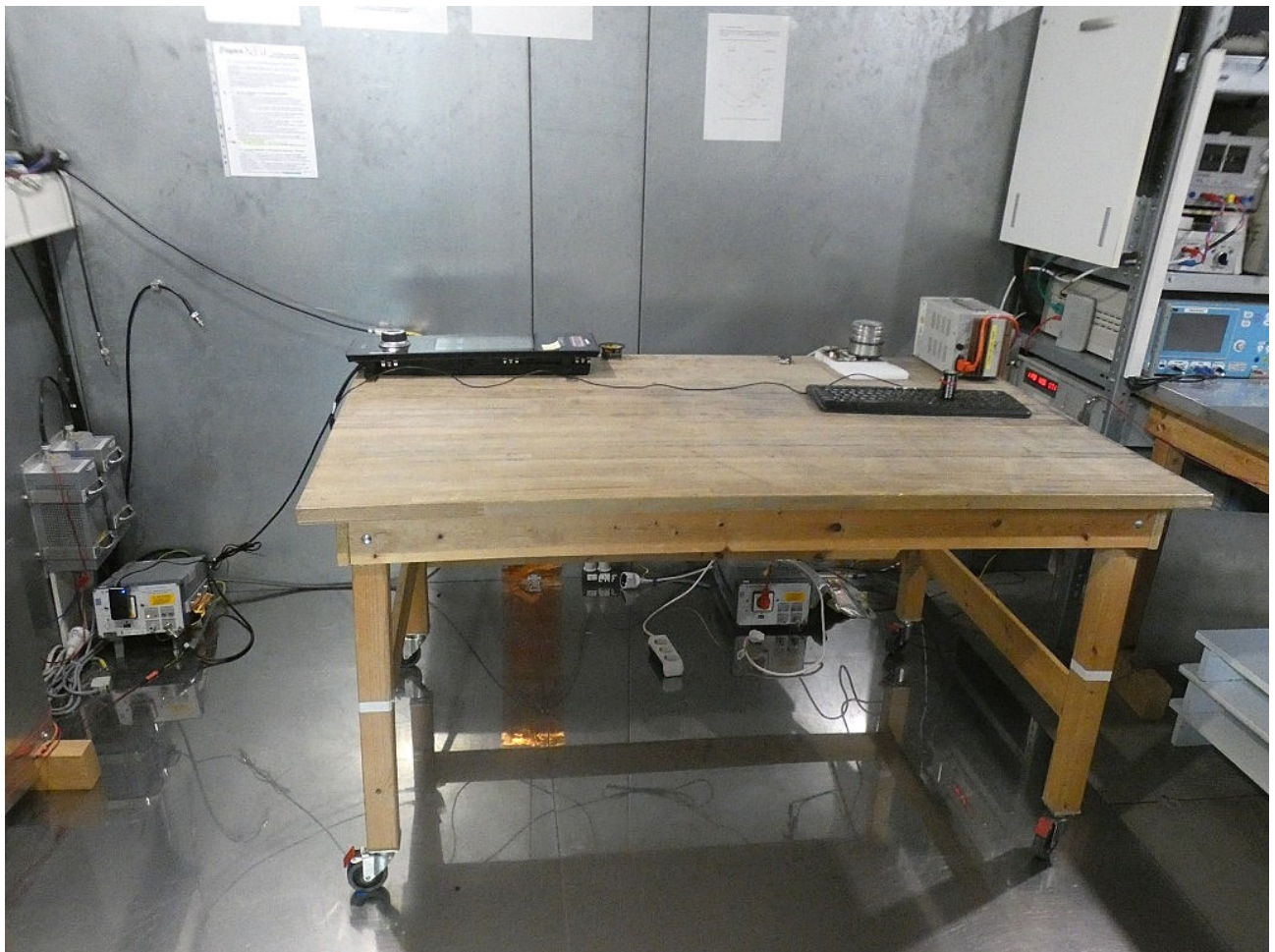
Photo 6: Test setup for conducted measurements (AC Port (power line), EUT supplied by auxiliary laboratory power supply, unintentional radiator §15, ANSI C63.4), setup with Switching Adapter (DE1183057ACDC1)
