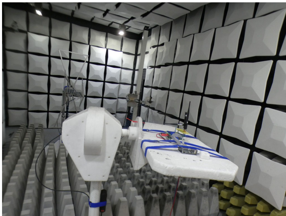
Photo 5: Test setup for radiated measurements above 1 GHz
