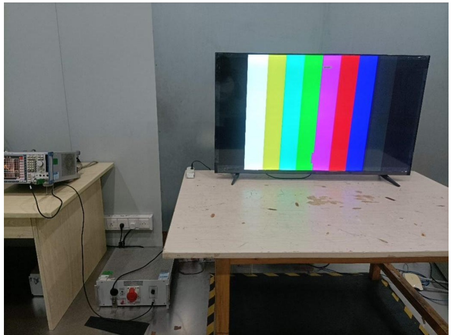
Conducted Emission Test Setup
