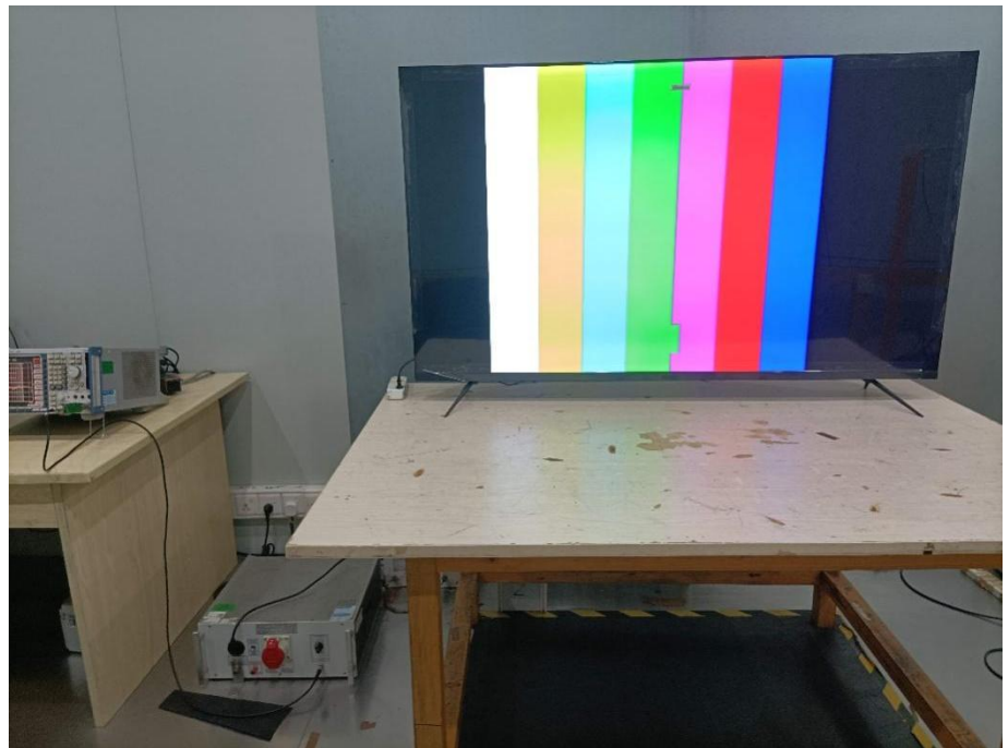
Conducted Emission Test Setup
