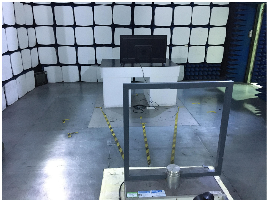
Radiation Emission Test Setup (Below 30MHz)
