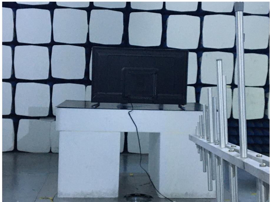
Radiation Emission Test Setup (30MHz to 1GHz)
