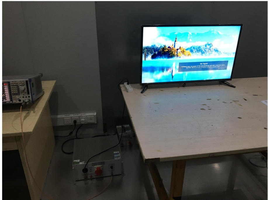
Conducted Emission Test Setup
