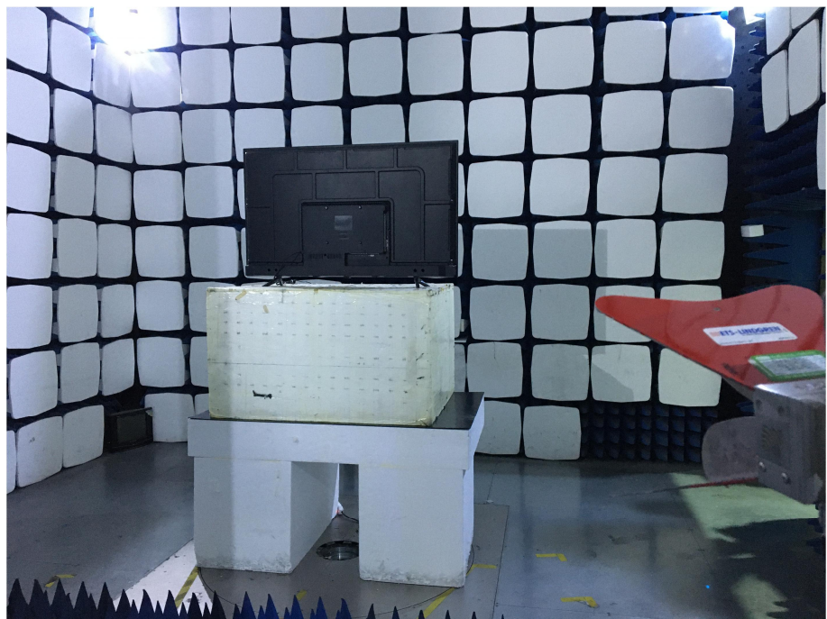
Radiation Emission Test Setup (1GHz to 18GHz)
