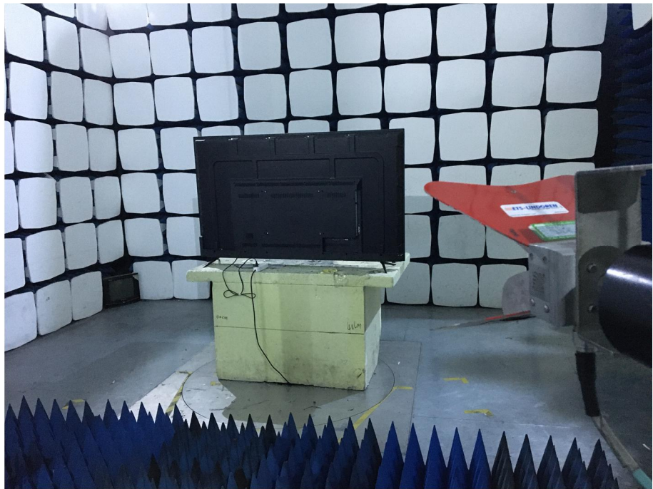
Radiation Emission Test Setup (1GHz to 18GHz)
