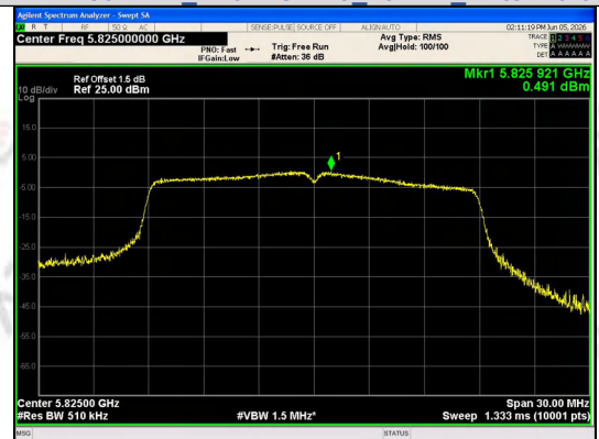
IEEE 802.11n Channel 165 20MHz Antenna 0
