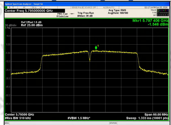
IEEE 802.11n Channel 159 40MHz Antenna 0
