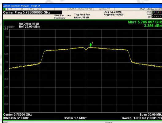
IEEE 802.11a_Channel 157_20MHz_Antenna 0
