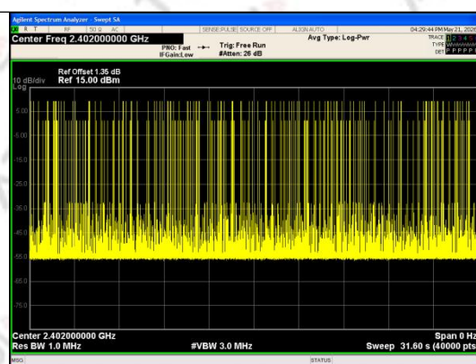
Number of Pulses in 31.6 seconds GFSK DH5
