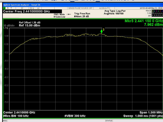
In-Band Reference Level \pi/4 DQPSK 2-DH5 Channel 39
