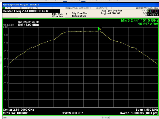
In-Band Reference Level GFSK DH5 Channel 39
