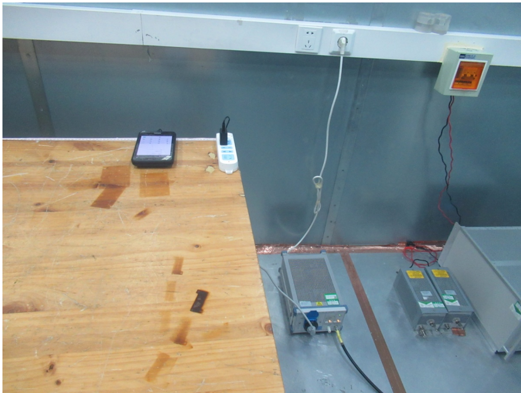
Picture 1: Conducted Emissions Test Setup
