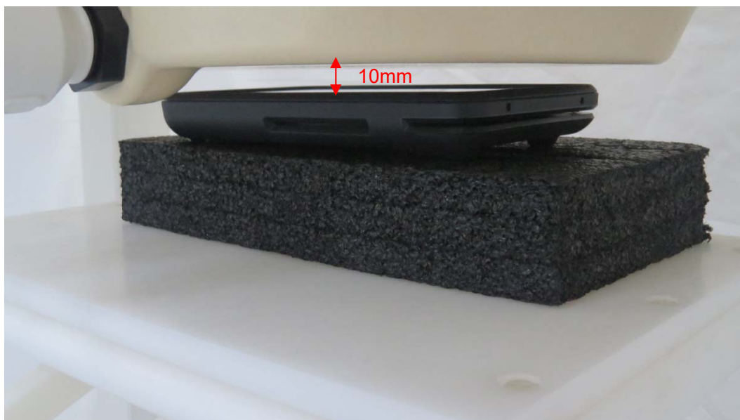
Picture 2: Front Side, the distance from handset to the bottom of the Phantom is 10mm
