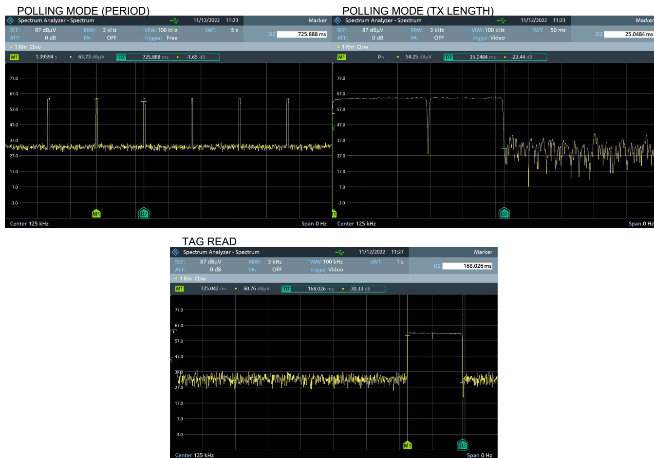
Figure 7: Example Pulsed Emission Characteristics (Duty Cycle).
