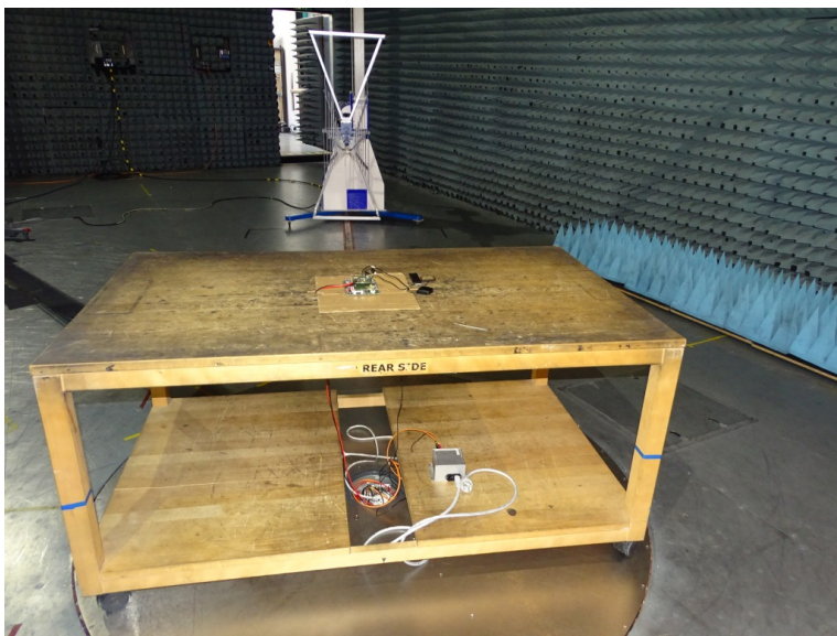
Photo 2: Test setup for radiated measurements
