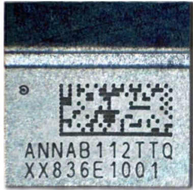
Figure 10: Product marking on the ANNA-B112 module
