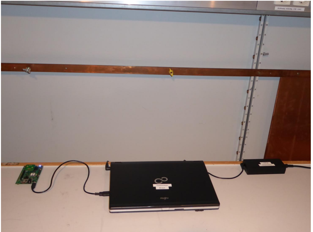
181323_SetMainsU1.JPG: Test setup mains conducted emissions; EVB-ANNA-B112U#117
