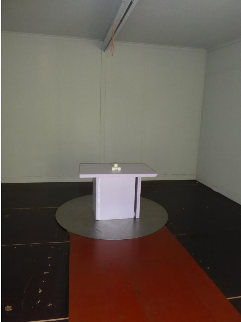
181323_SetRadU9.JPG: Test setup open area test site; EVB-ANNA-B112U#117, 30 MHz – 1 GHz
