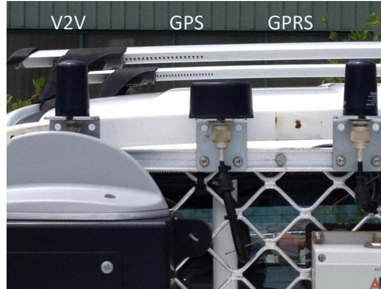
Note: Antenna Spacing between V2V and GPRS should be a minimum of 300mm.
