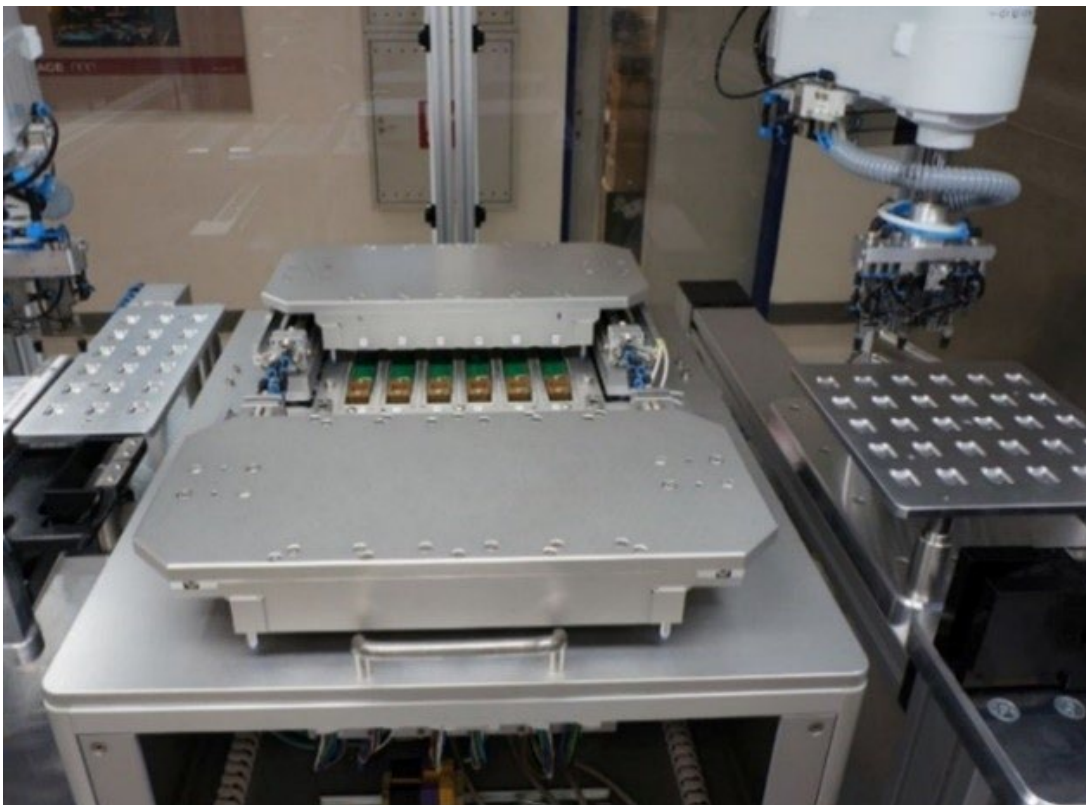
Figure 14: Automatic test equipment for module test
