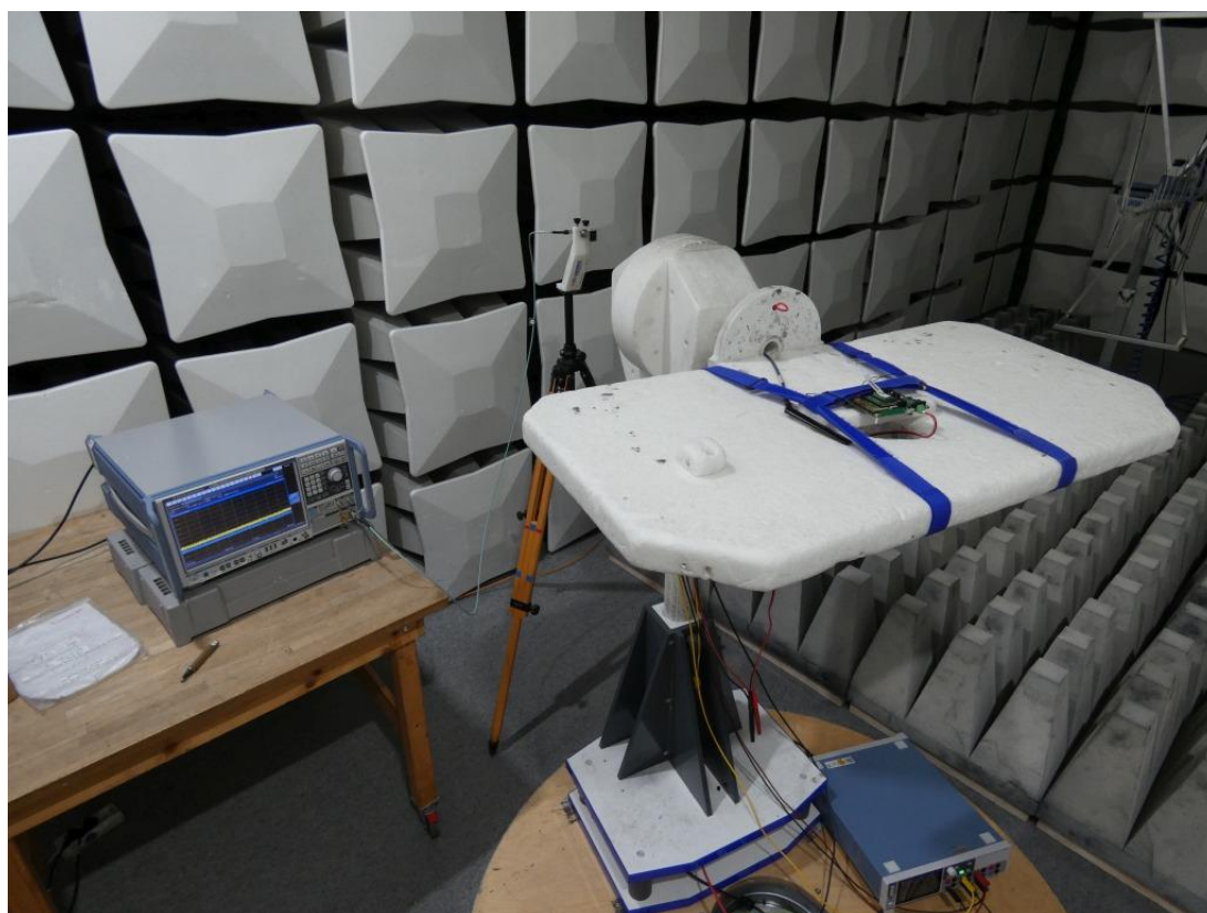
Photo 4: Test setup for radiated measurements above 26 GHz
