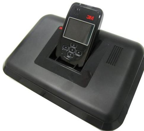
Figure 5: Two-Piece Unit docked in GPS Base Unit
