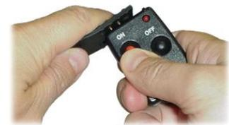
The red LED on the MRD turns on for 2 seconds and then flashes for another 2 seconds. The flashing indicates that the RF Transmitter has passed the first phase of its activation.
