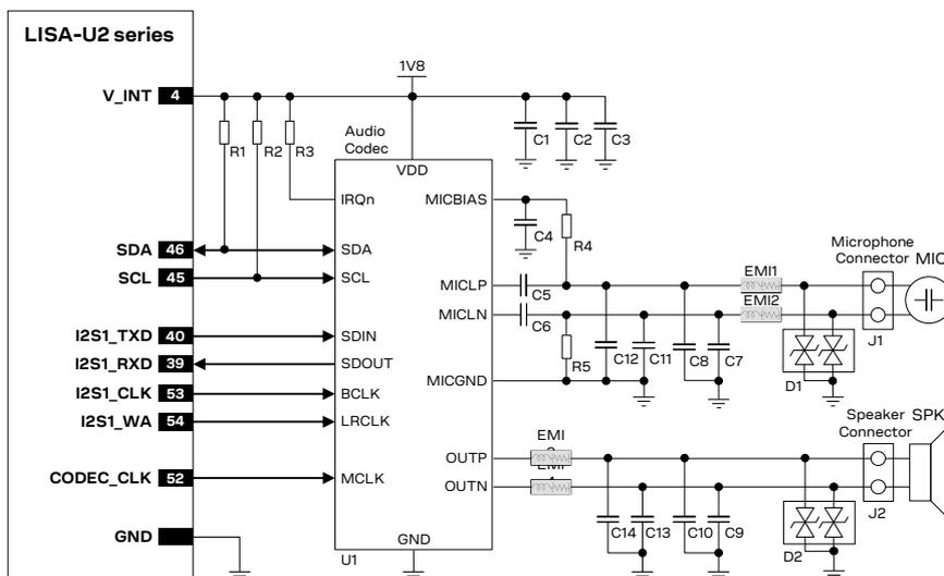
Figure 50: I<sup>2</sup>S interface application circuit with an external audio codec to provide voice capability
