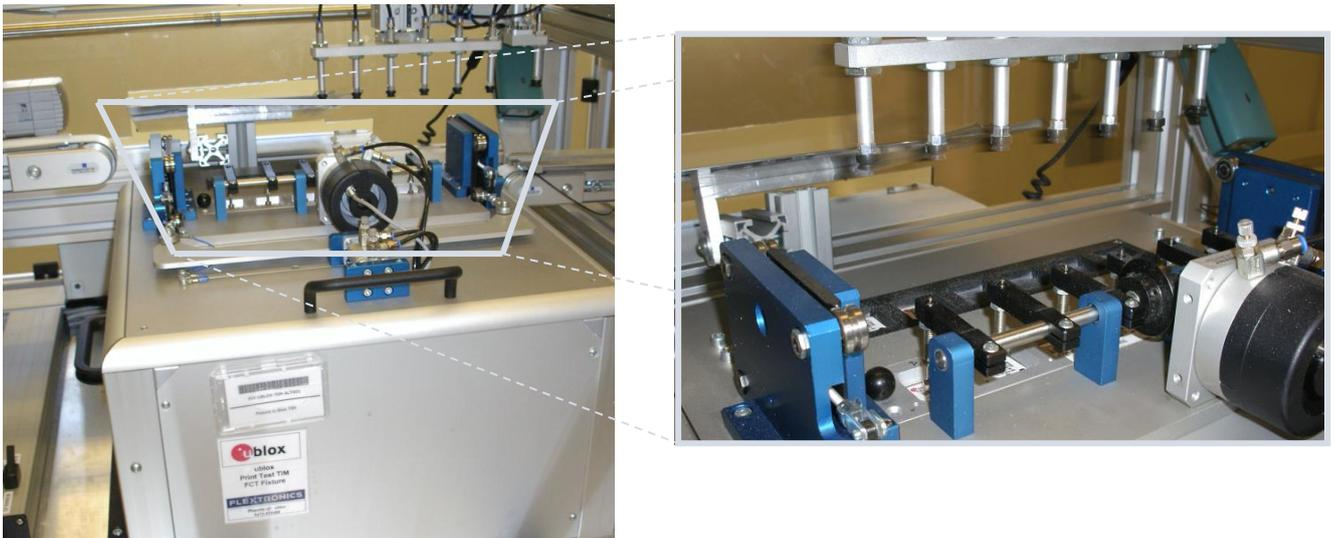
Figure 75: Automatic test equipment for module tests
