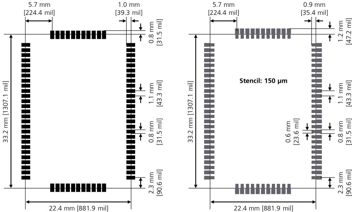
**Figure 61: LISA-U2 modules suggested footprint and paste mask**
