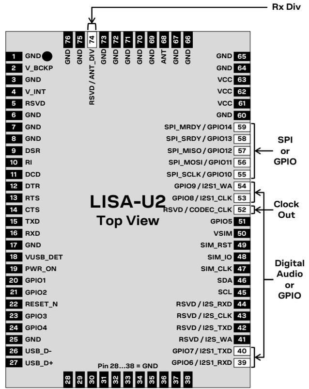
Figure 78: LISA-U2 series pin assignment (highlighted name/function changes)
