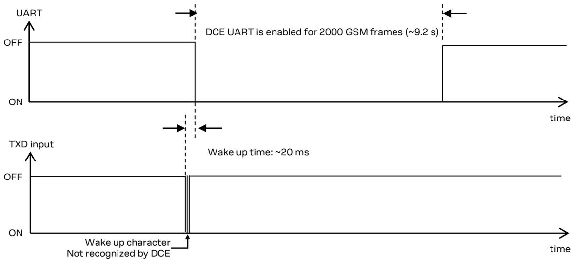
Figure 29: Wake-up via data reception without further communication
