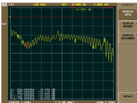
Figure 64:  $|S_{11}|$  sample measurement of a wideband antenna
