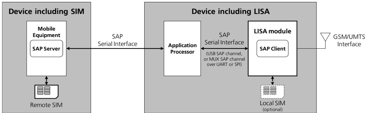
**Figure 70: Remote SIM access via completely wired connection**
