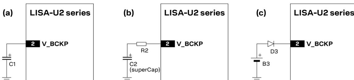
Figure 16: Real time clock supply (**V\_BCKP**) application circuits: (a) using a 100 μF capacitor to let the RTC run for ~50 s after **VCC** removal; (b) using a 70 mF capacitor to let RTC run for ~10 hours after **VCC** removal; (c) using a non-rechargeable battery
