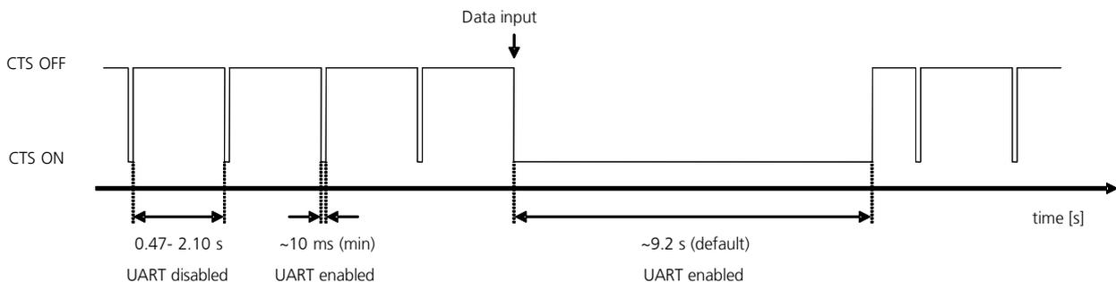
**Figure 28: CTS behavior with power saving enabled (AT+UPS<sub>V</sub>=1) and HW flow control enabled: the CTS output line indicates when the UART interface of the module is enabled (CTS = ON = low level) or disabled (CTS = OFF = high level)**
