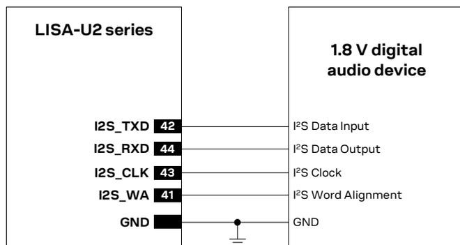
Figure 49: I<sup>2</sup>S interface application circuit with a generic digital audio device
