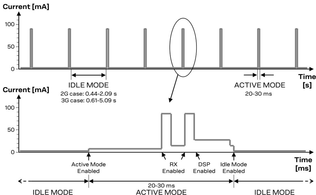
**Figure 14: Description of VCC current consumption profile versus time when the module is registered with 2G or 3G networks: the module is in idle mode and periodically wakes up to active mode to monitor the paging channel for paging block reception**
