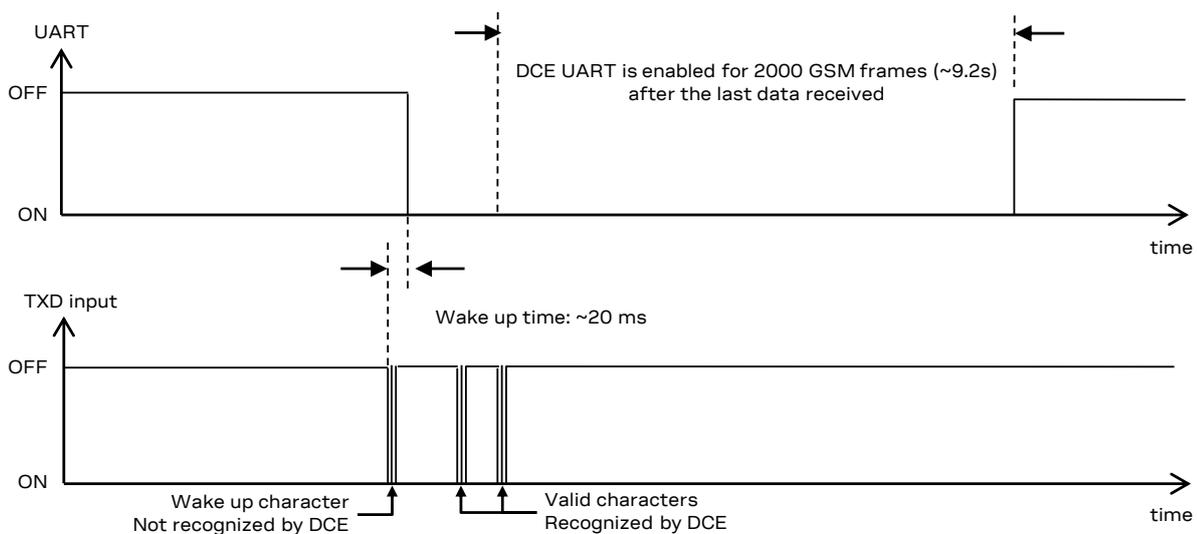
Figure 30: Wake-up via data reception with further communication
