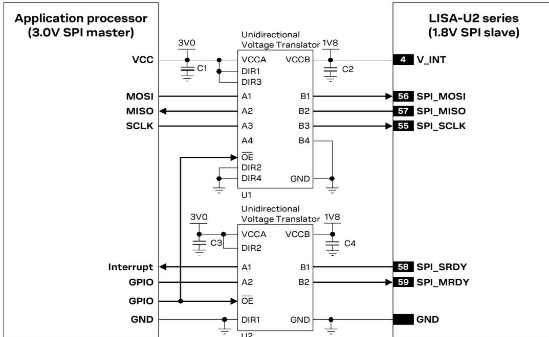
**Figure 46: IPC / SPI Interface application circuit connecting LISA-U2 series 1.8V SPI slave to a 3.0 V SPI master**
