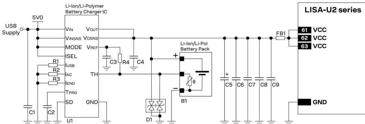
Figure 10: Li-Ion (or Li-Polymer) battery charging application circuit
