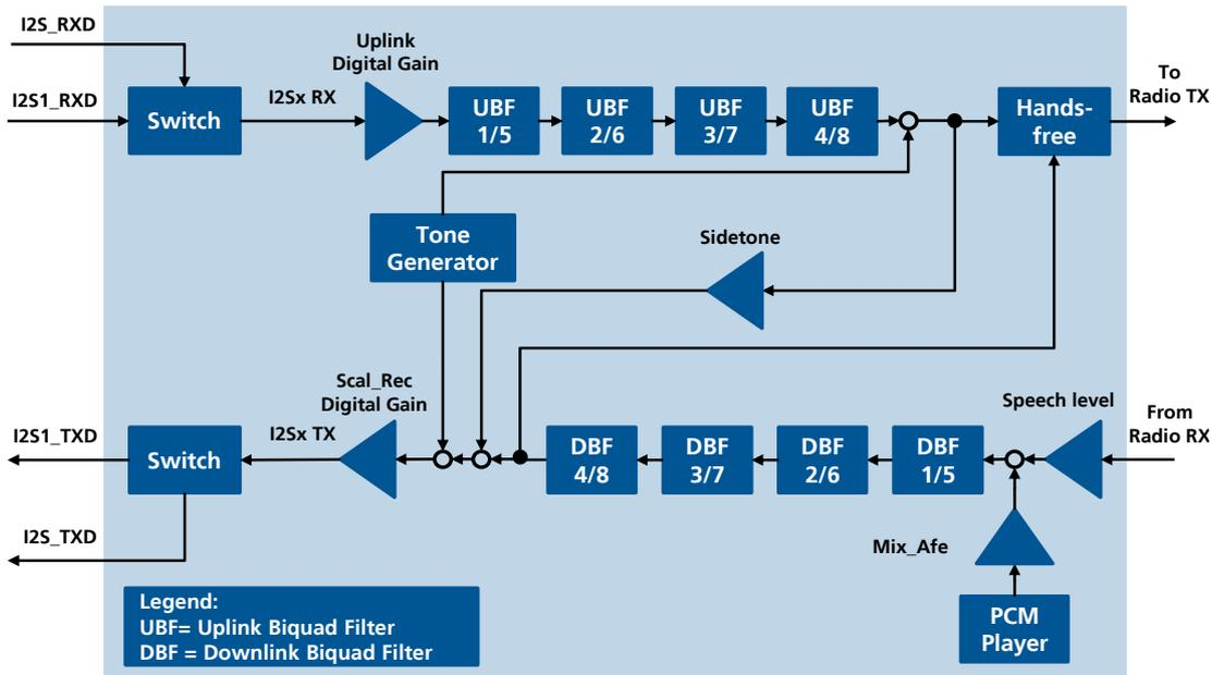
Figure 51: Audio processing system of LISA-U2 series modules
