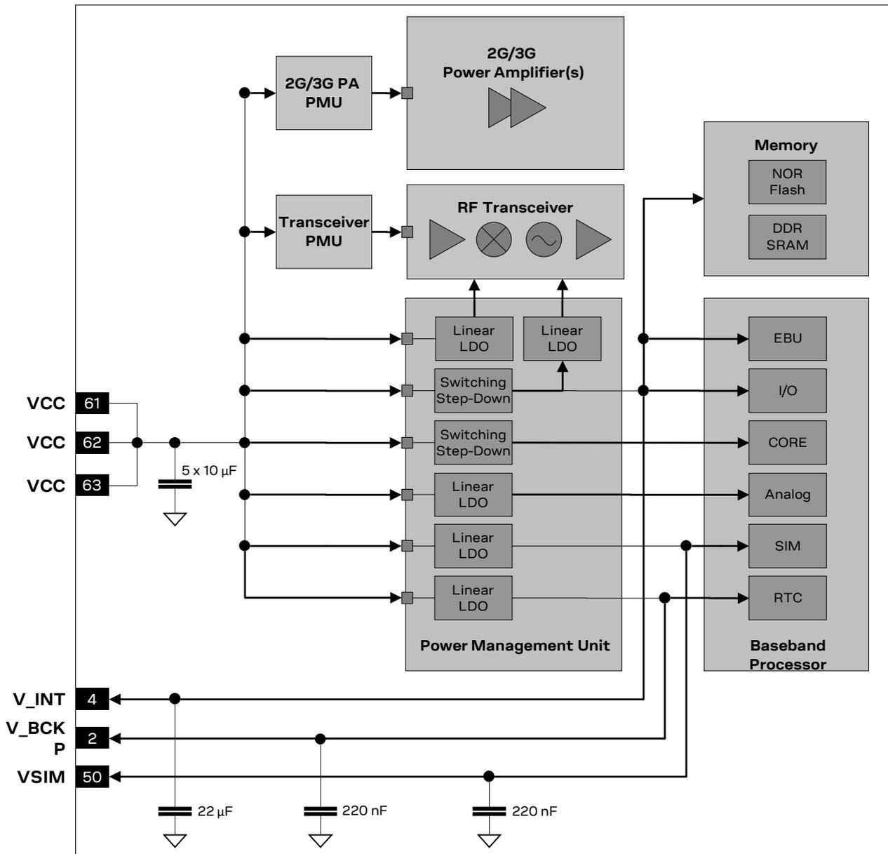
Figure 3: LISA-U2 series power management simplified block diagram
