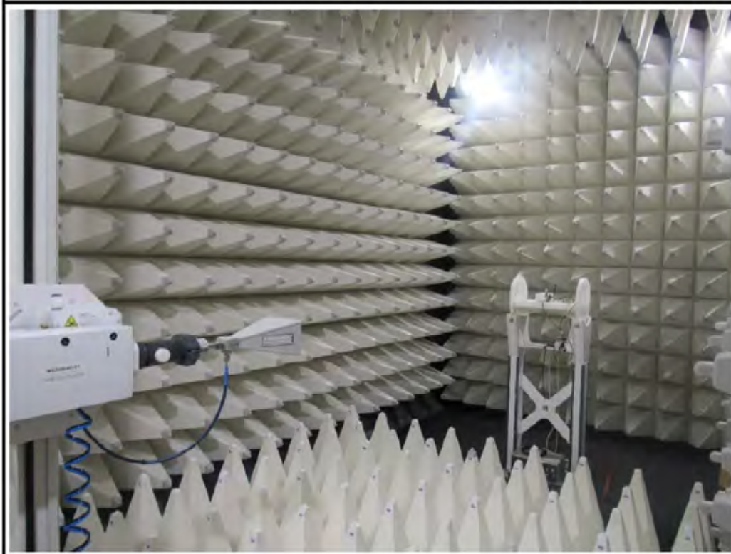
Setup for measurements above 1 GHz (1)
