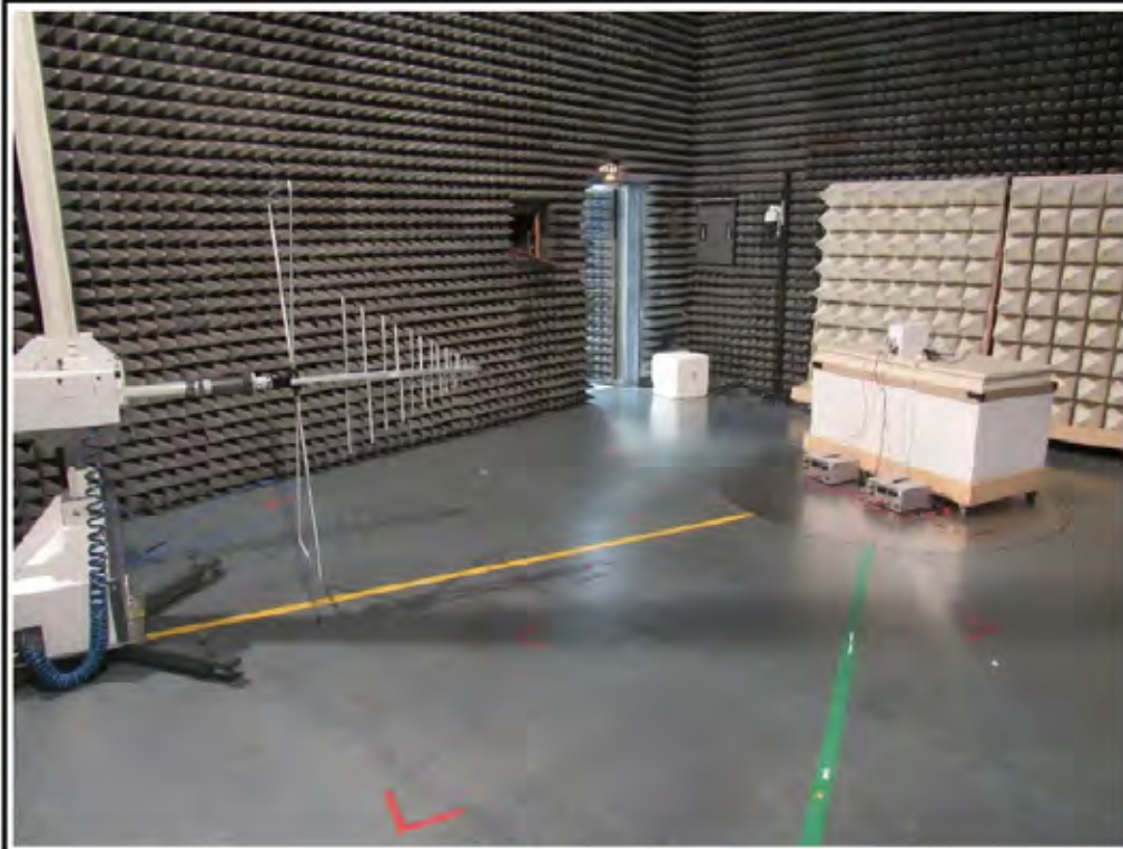
Setup for measurements below 1 GHz (2)
