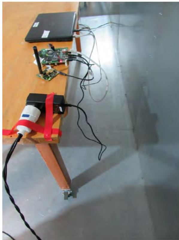
Setup for measurements 150 kHz - 30 MHz (cables)
