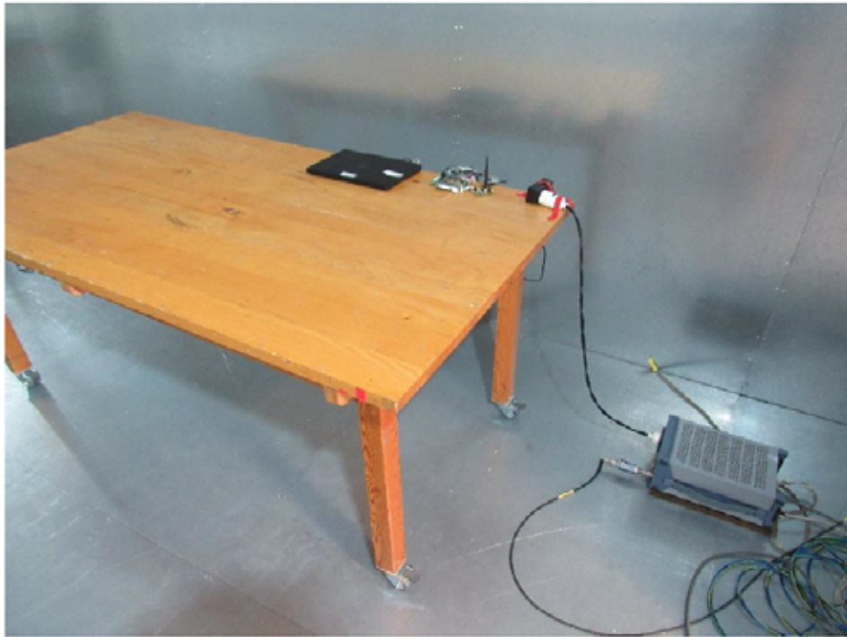
Setup for measurements 150 kHz - 30 MHz
