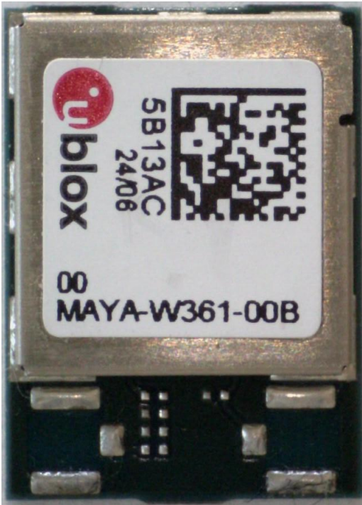
Figure 1: MAYA-W361-00B top view external photo
