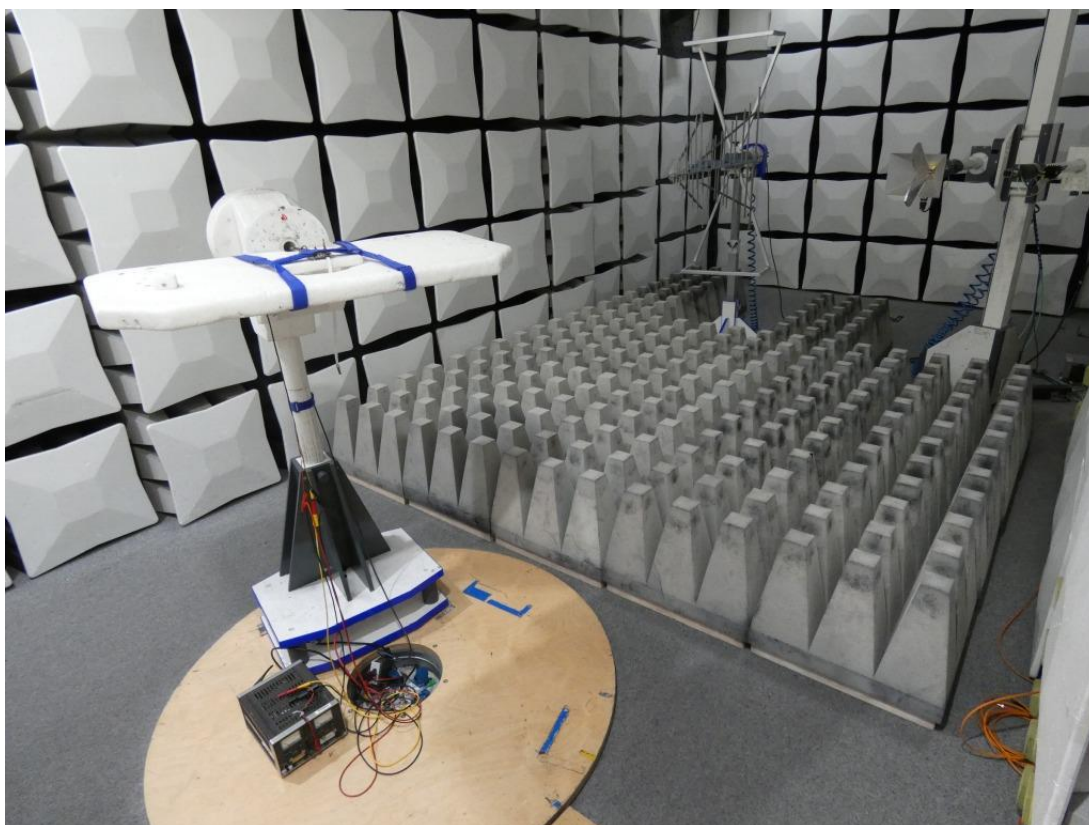
Photo 3: Test setup for radiated measurements above 1 GHz
