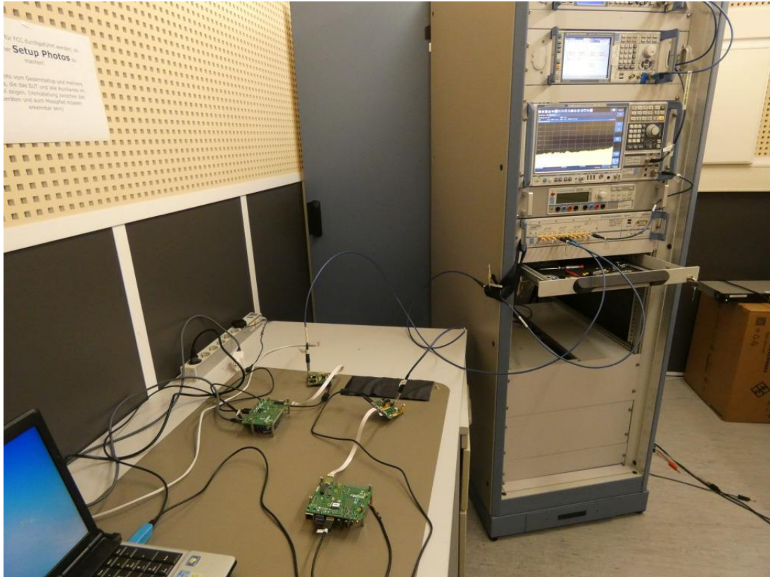
Photo 9: Test Setup for Contention Based Protocol
