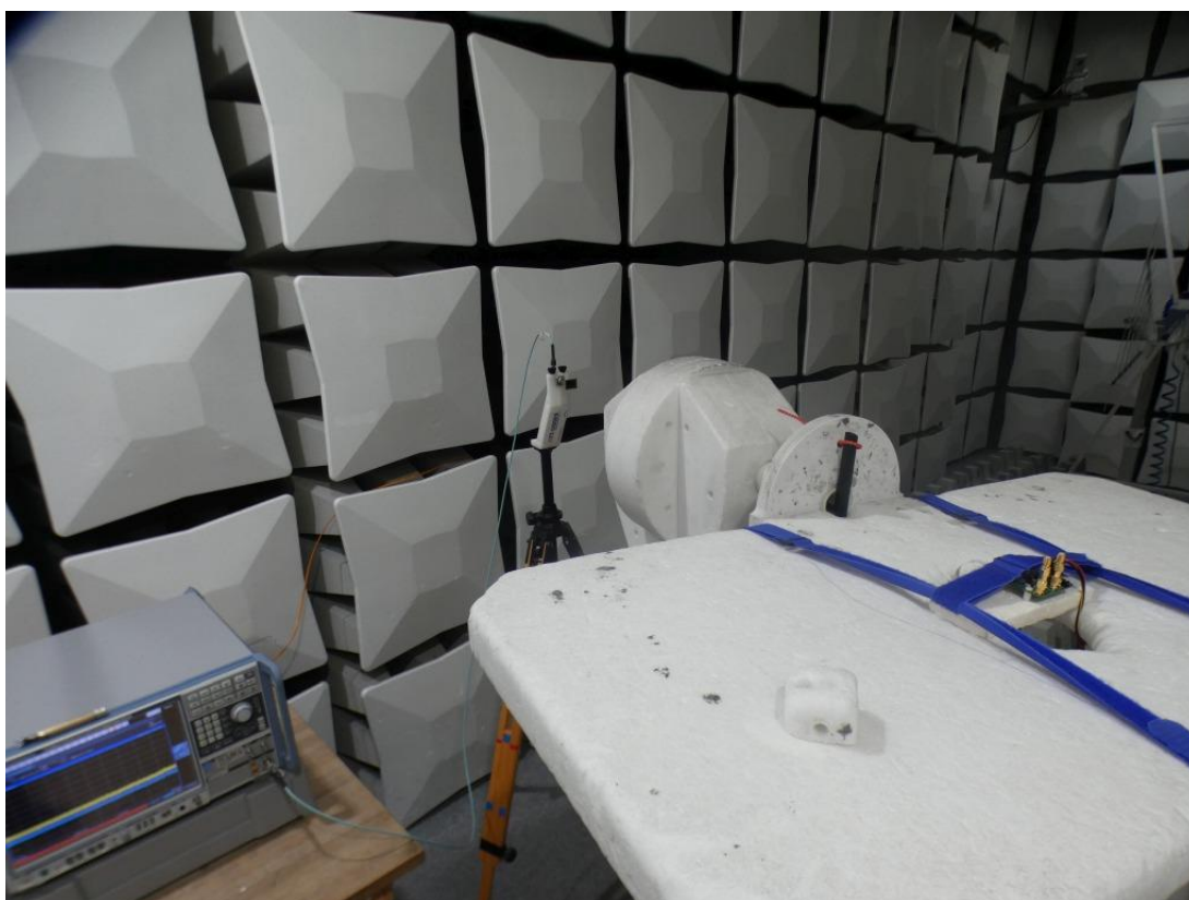
Photo 4: Test setup for radiated measurements above 26 GHz
