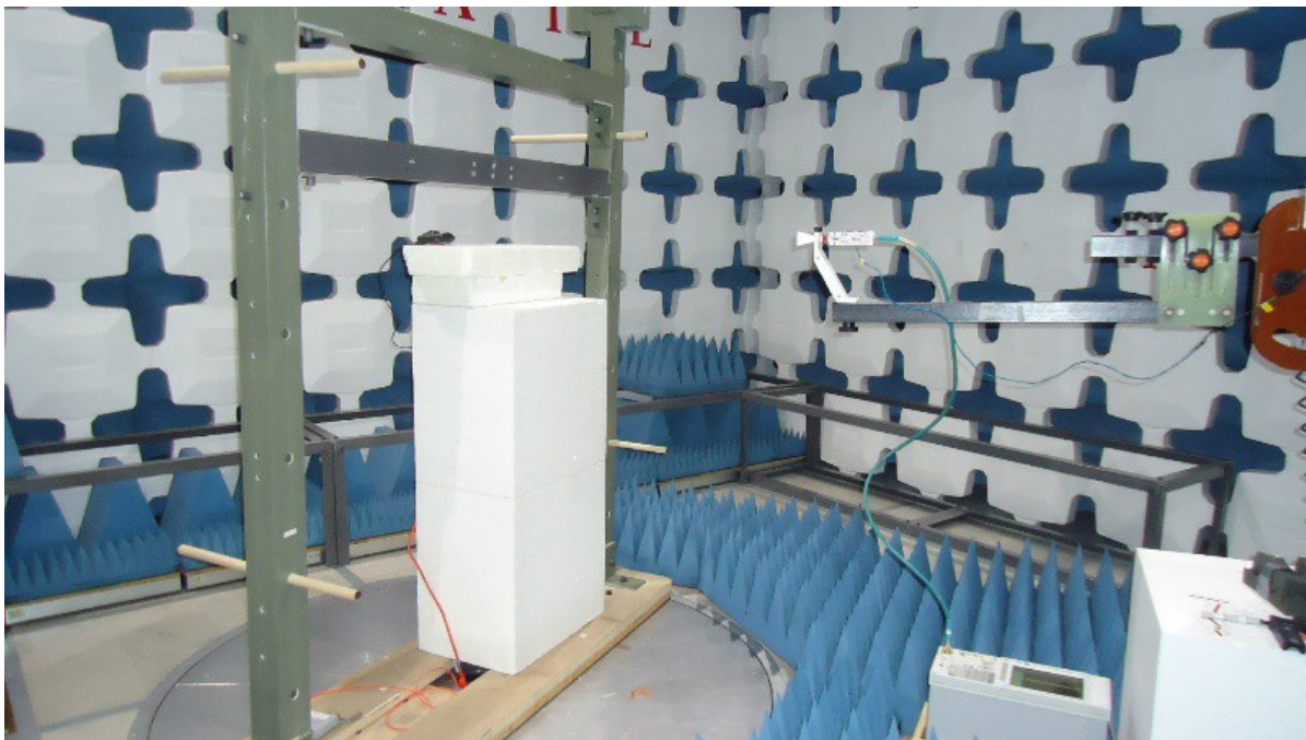
Figure 4.9 - Radiated Emission Test Setup - Side View
