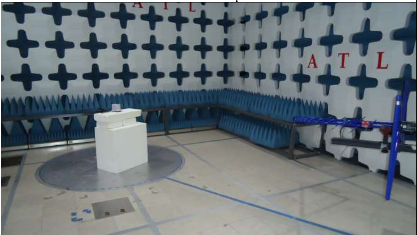
Radiated Emission Test Setup - Side View
