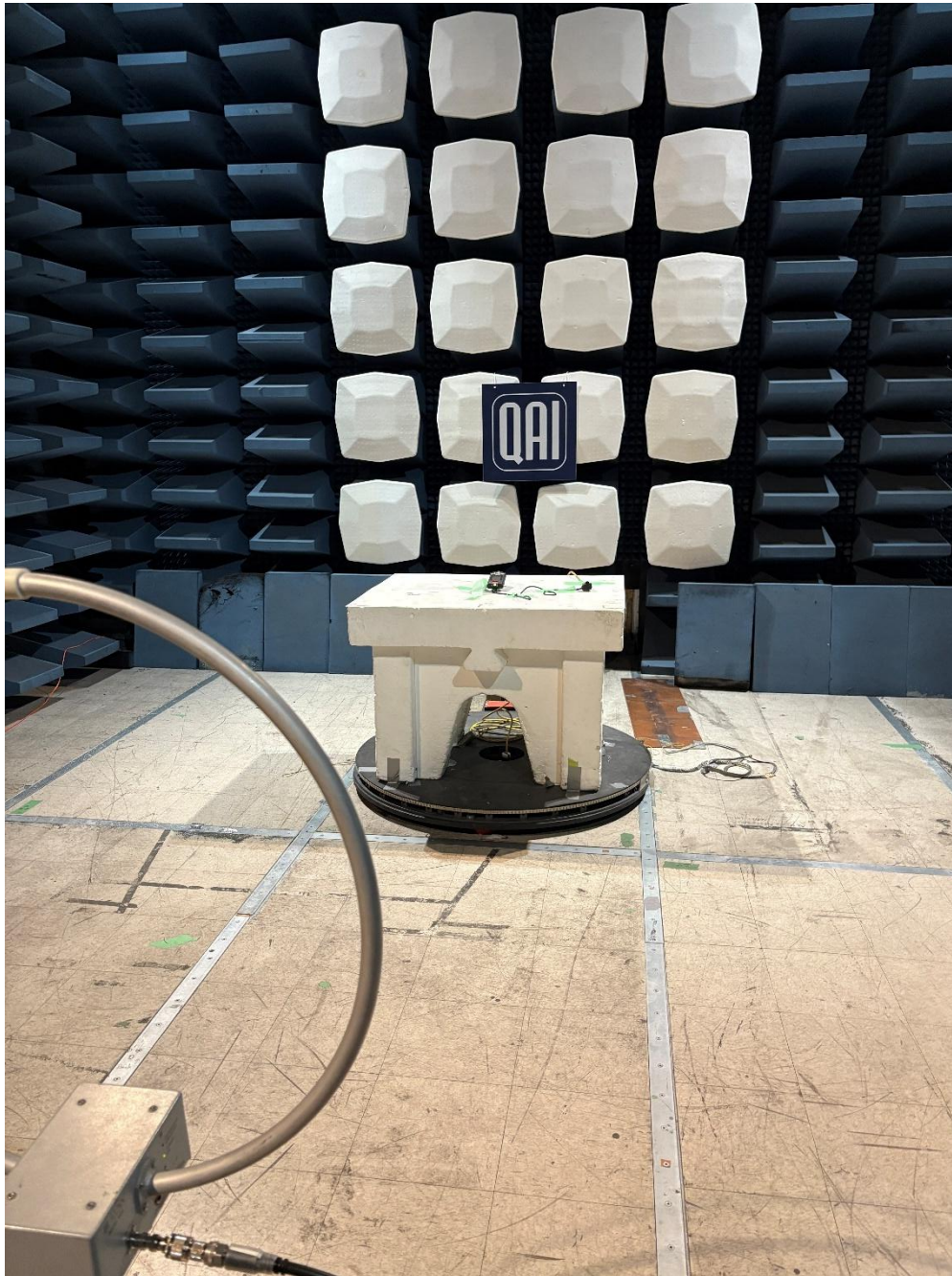
Figure 2: Radiated Emissions – 10kHz to 30MHz
