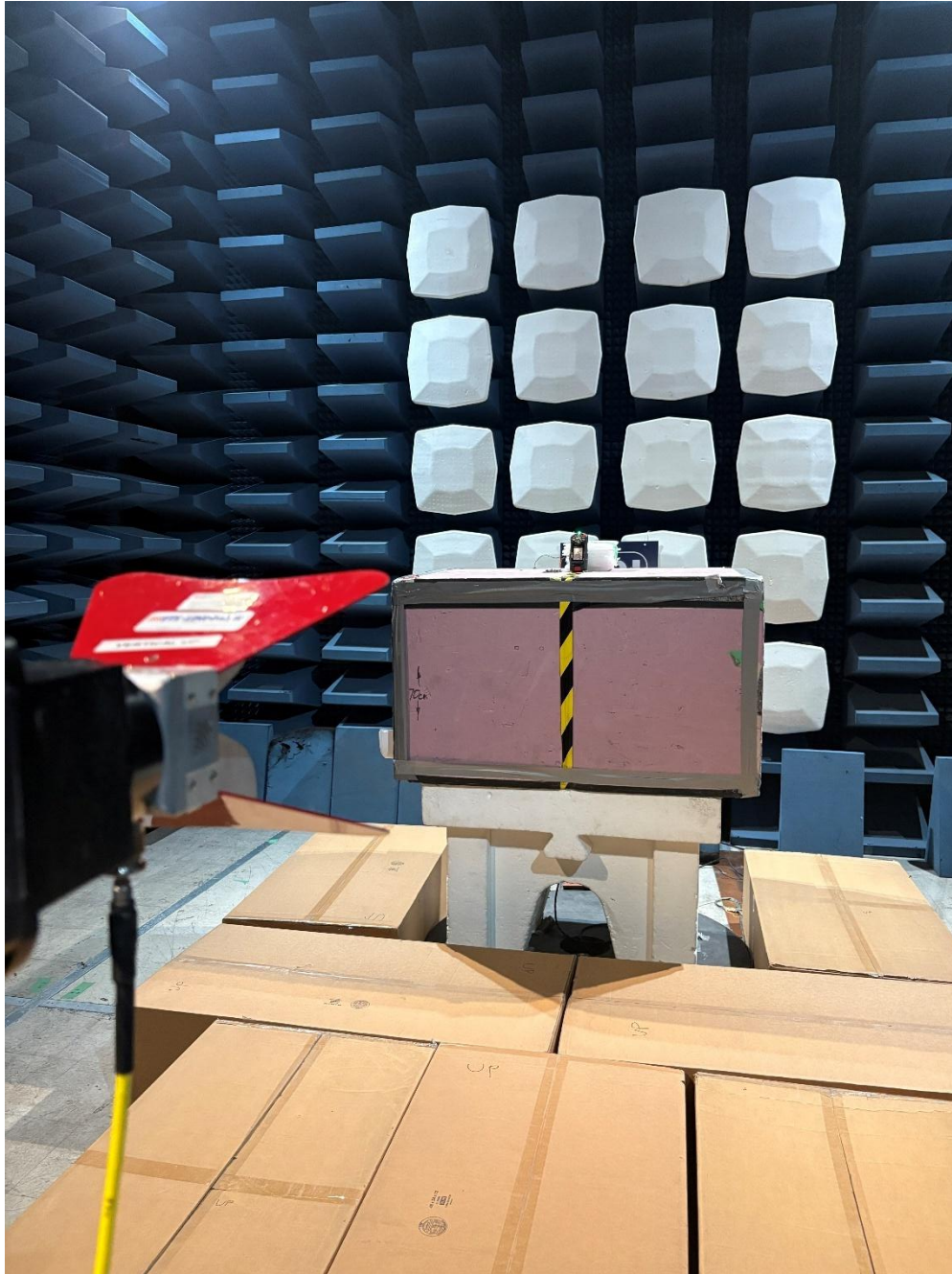
Figure 3: Radiated Emissions – 10kHz to 30MHz
