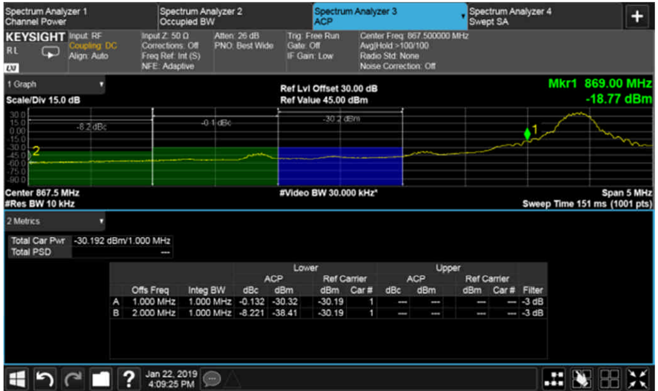
Plot of lower band edge for Low channel
