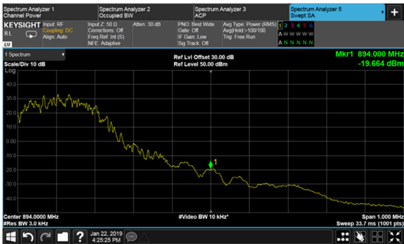
Plot of upper band edge for High channel, 3kHzRBW
