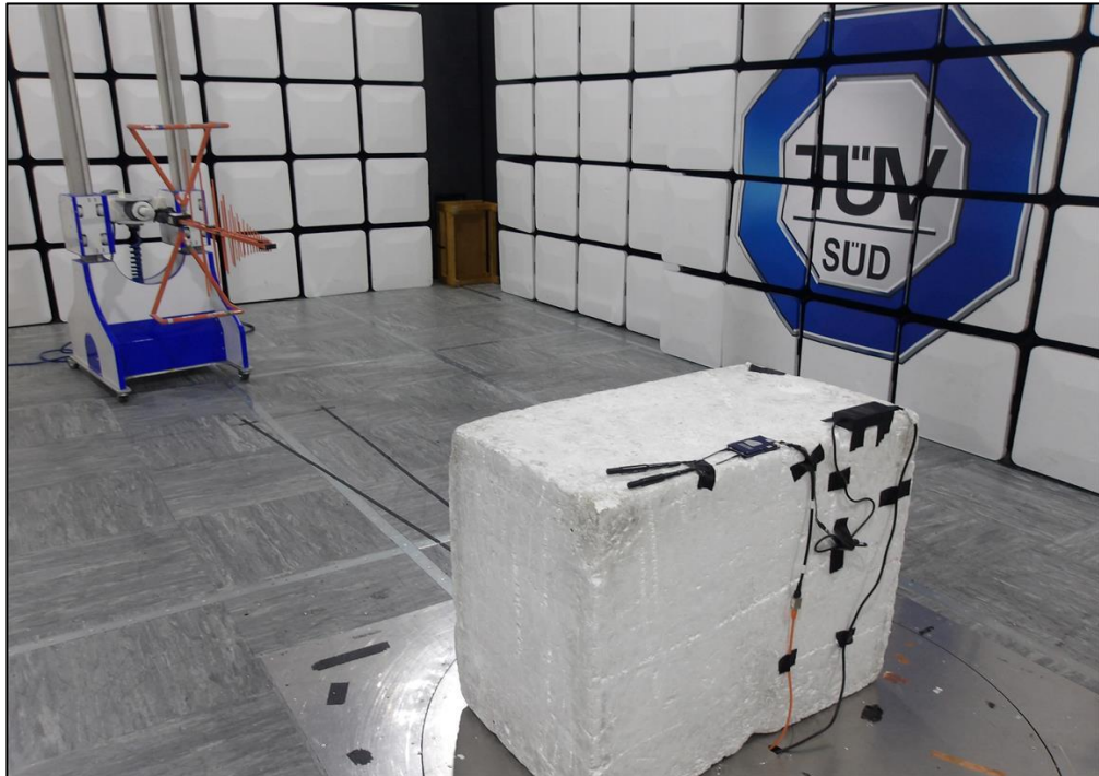
Figure 19 - Test Setup - 30 MHz to 1 GHz
