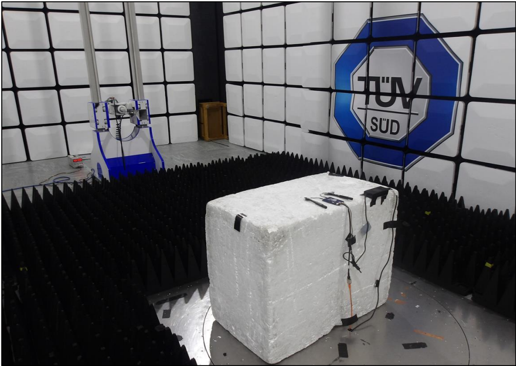
Figure 21 - Test Setup - 8 GHz to 15 GHz
