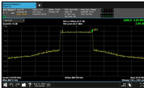
Figure 40 - B (B) 2437.5 MHz (CH5002) 99% Bandwidth
