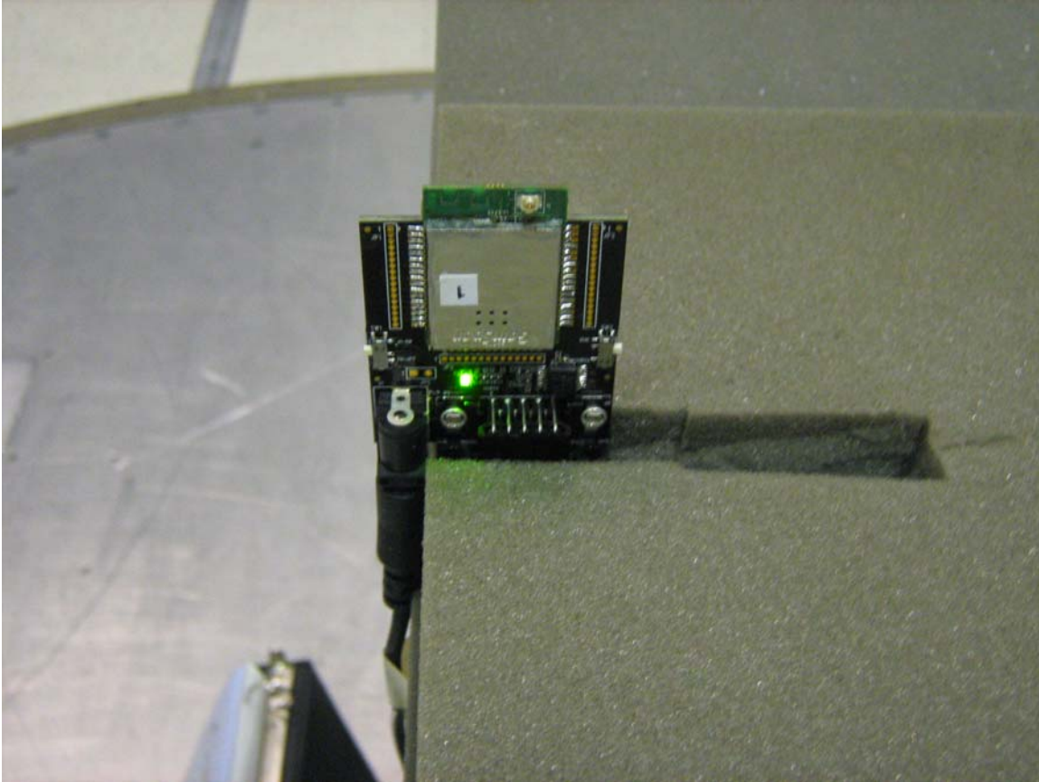
Figure 9: Radiated Emission Setup on Z-Axis
