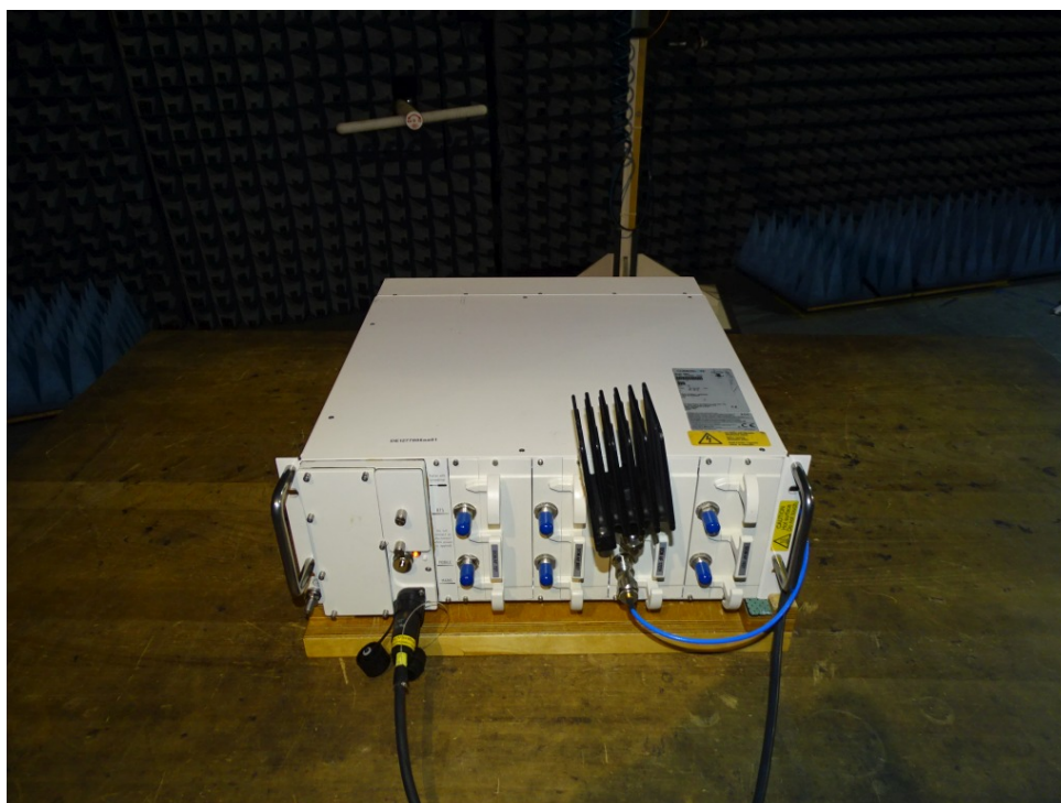
Photo 2: Test setup for radiated emissions measurements in semi-anechoic chamber (30 MHz to 1 GHz), detailed view (front side)
