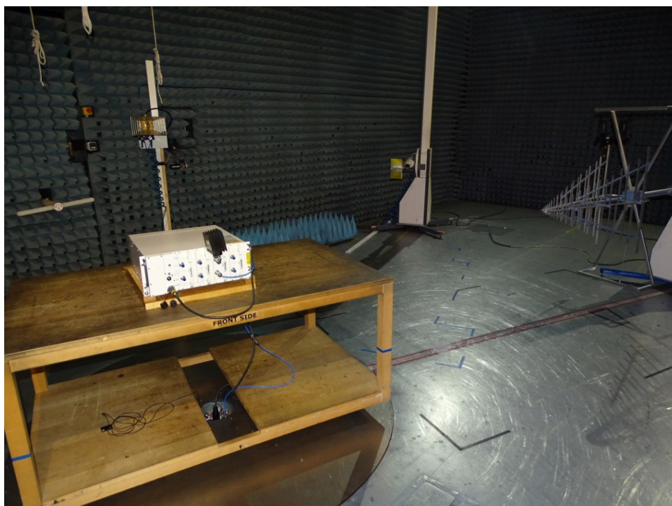
Photo 1: Test setup for radiated emissions measurements in semi-anechoic chamber (30 MHz to 1 GHz), right side view
