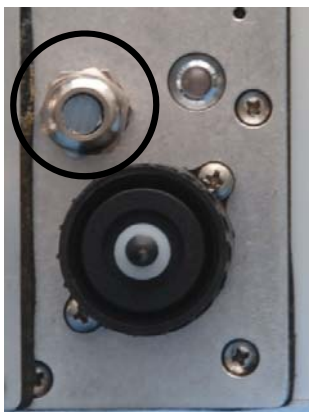
figure 4-12 External cable gland
