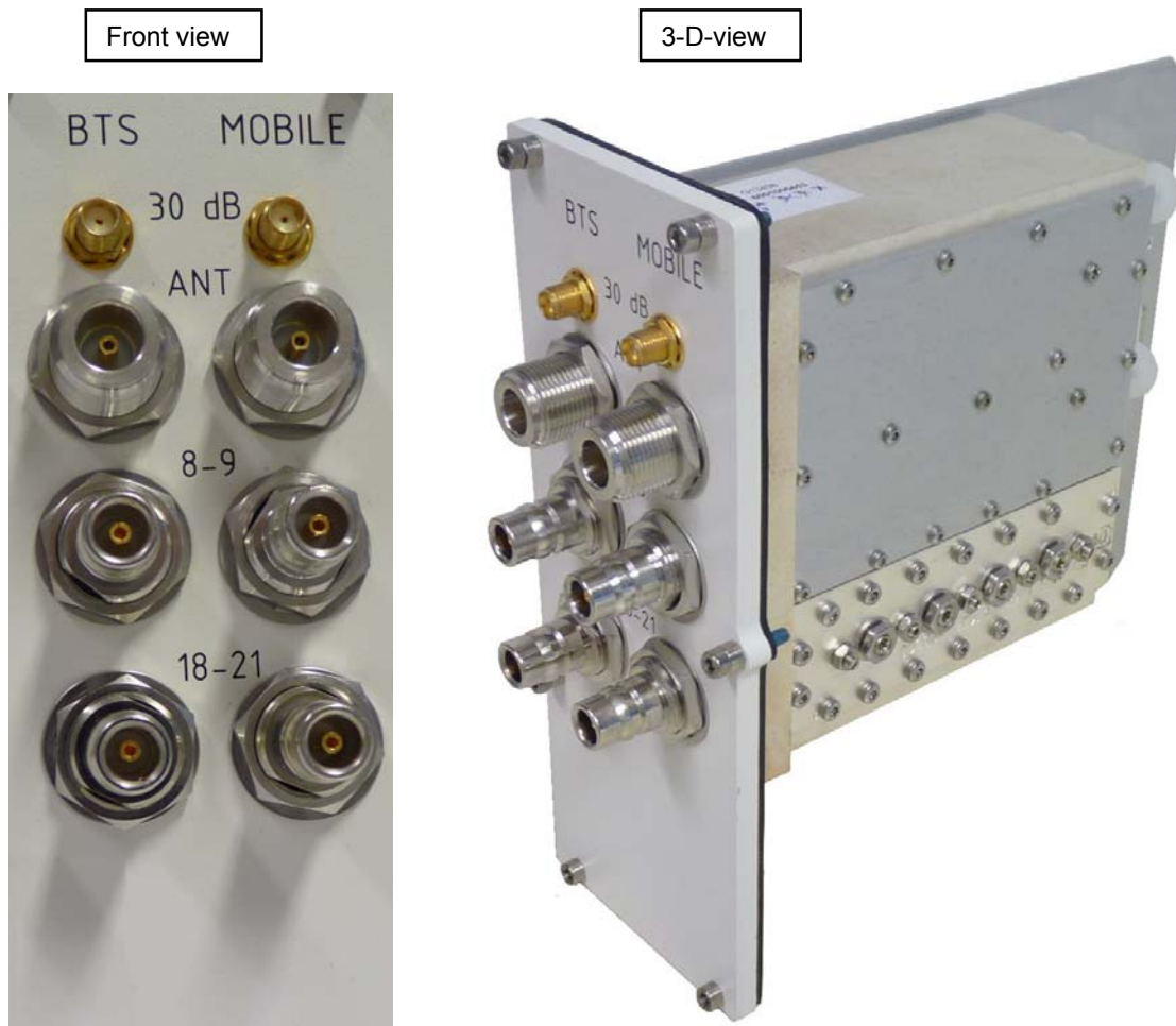
figure 4-3 Node AM4 2-band combiner (800-900 and 1800-2100 MHz) with two pairs of band ports
