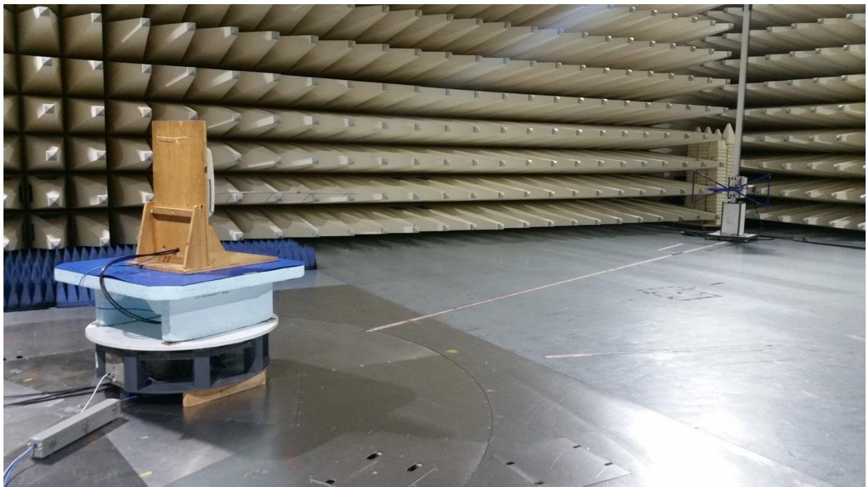
picture 8.2: Test setup: Field Strength Emission <1 GHz @10m in the SAC
