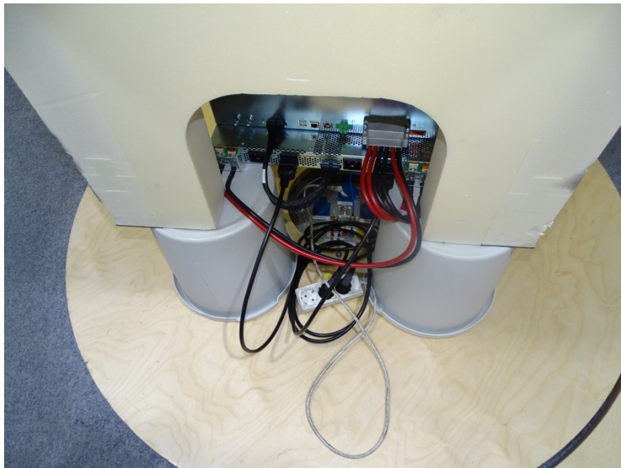
Photo 4: Test setup for radiated emissions measurements in fully-anechoic chamber (1 GHz to 22 GHz), front side view (auxiliary equipment below table)
