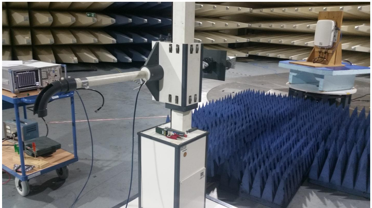
Test setup: Field Strength Emission 18 – 26,5 GHz @3m in the SAC
