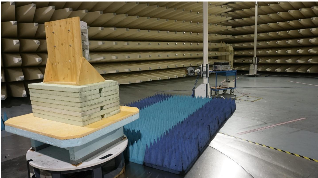
Photograph 7: Setup of radiated emissions measurement in the frequency range from 18 GHz to 27 GHz.
