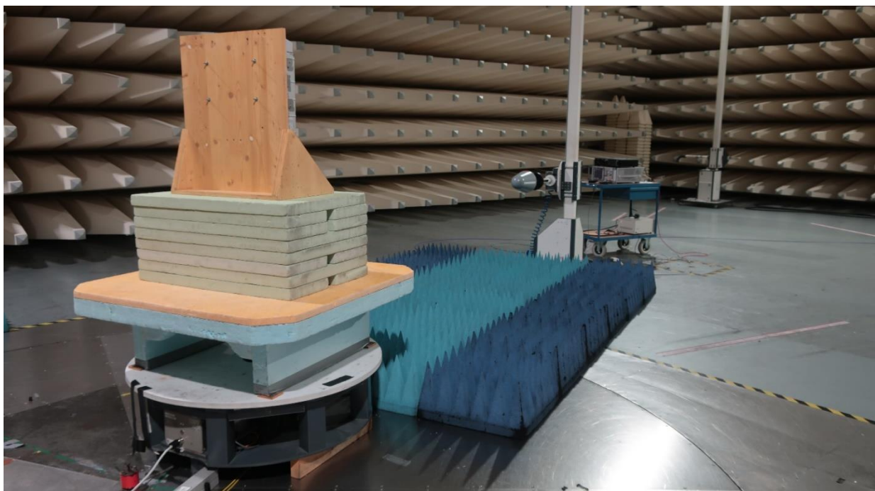
Photograph 5: Setup of radiated emissions measurement in the frequency range from 1 GHz to 18 GHz.
