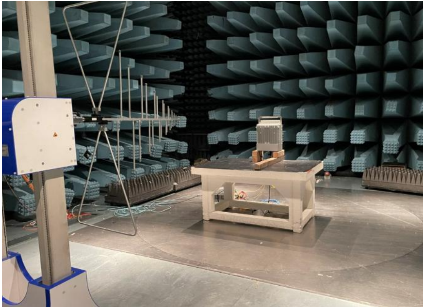
Figure-3: Radiated emissions set-up for frequencies below 1 GHz
