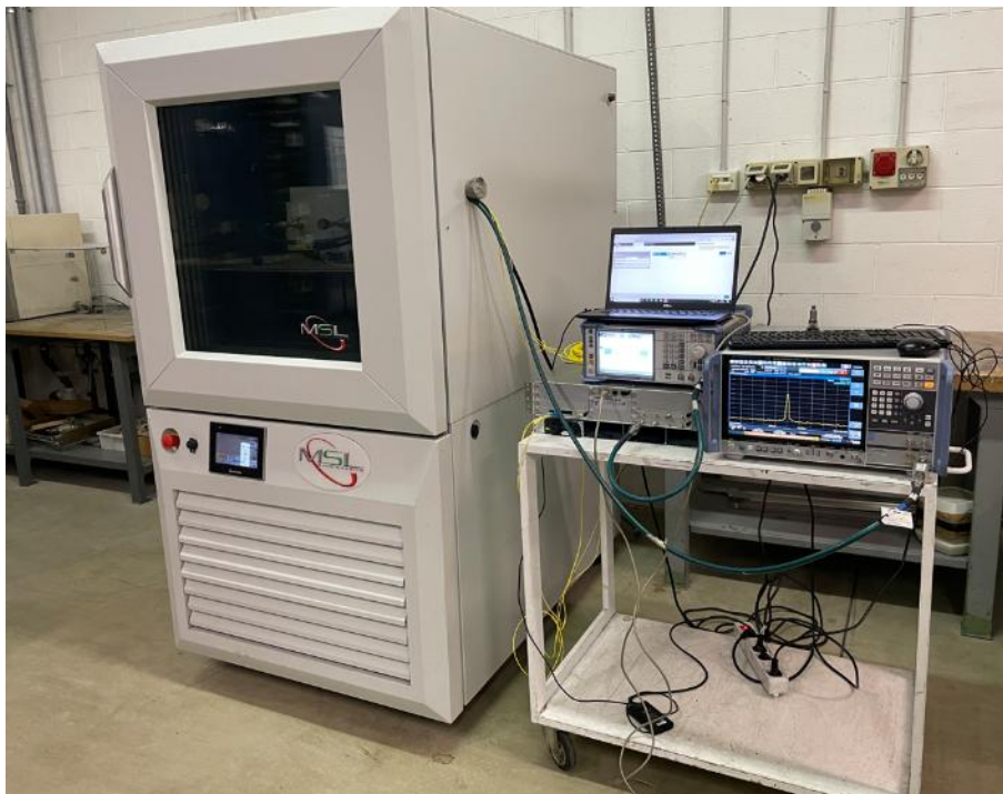
Figure-2: Antenna port testing set-up in climatic chamber
