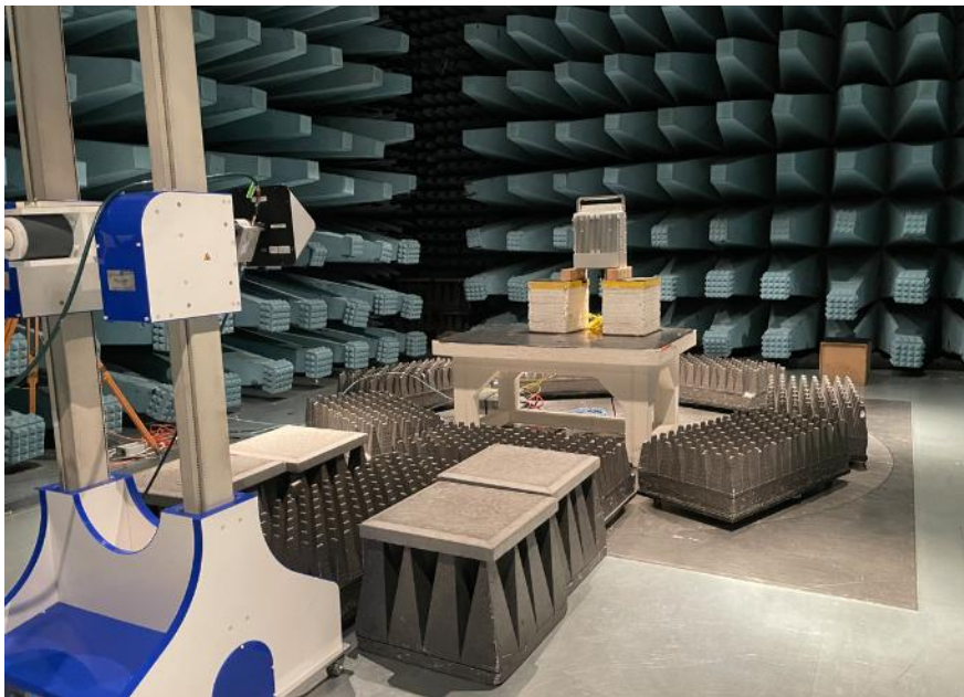
Figure-4: Radiated emissions set-up for frequencies above 1 GHz
