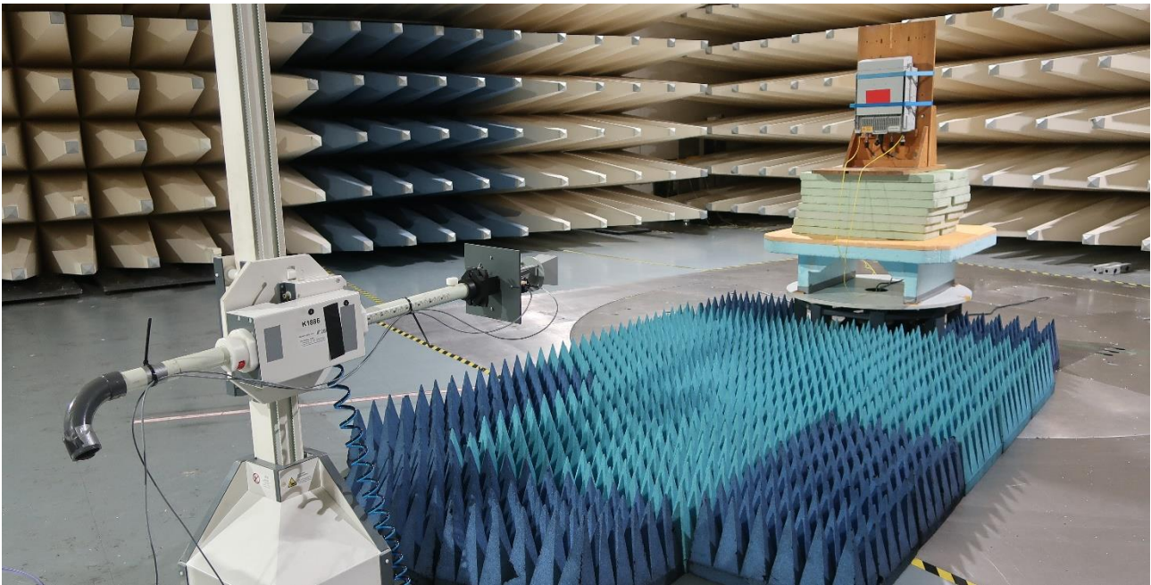
Photograph 6: Setup of radiated emissions measurement in the frequency range from 18 GHz to 26 GHz.
