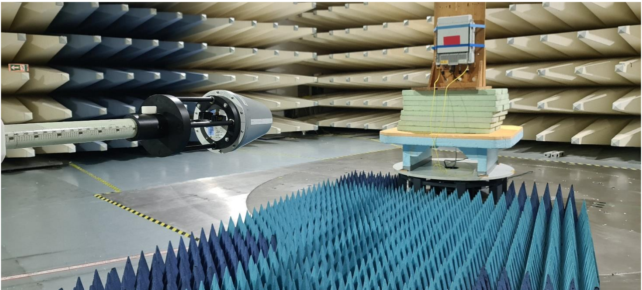
Photograph 4: Setup of radiated emissions measurement in the frequency range from 1 GHz to 18 GHz.
