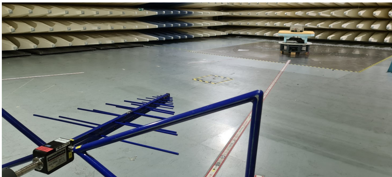
Photograph 7: Setup of radiated emissions measurement in the frequency range 30 – 1000 MHz
