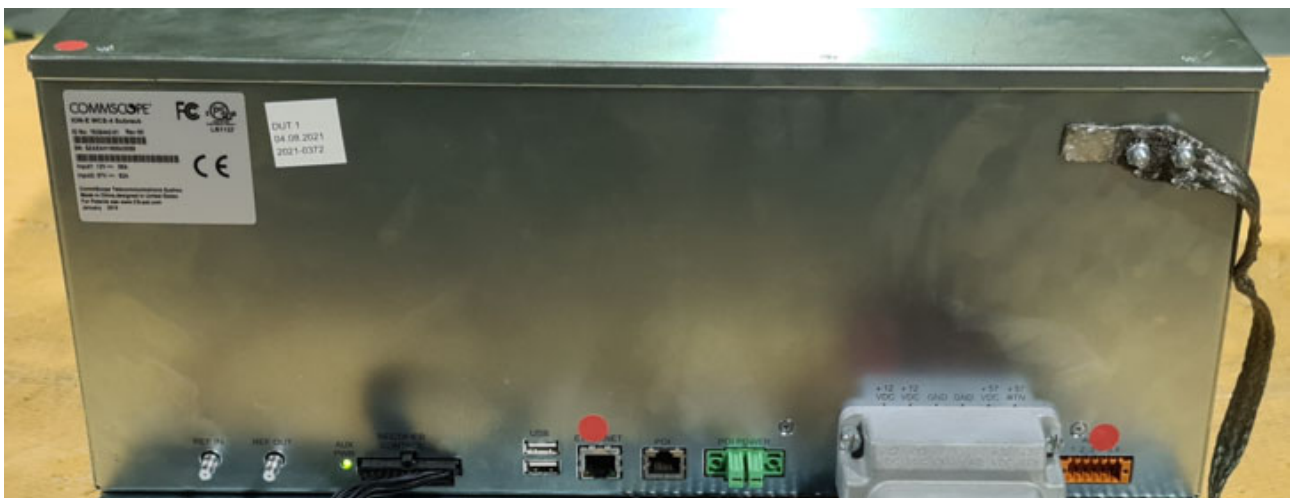
Photograph 6: Photograph of DUT's grounding
