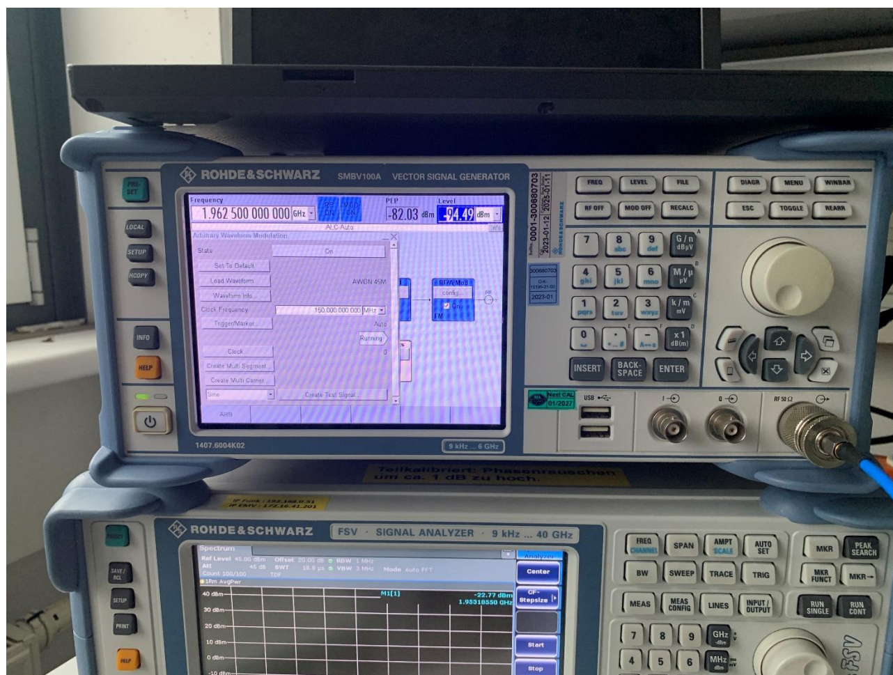
Photograph 1: Generator Type SMBV100A.
