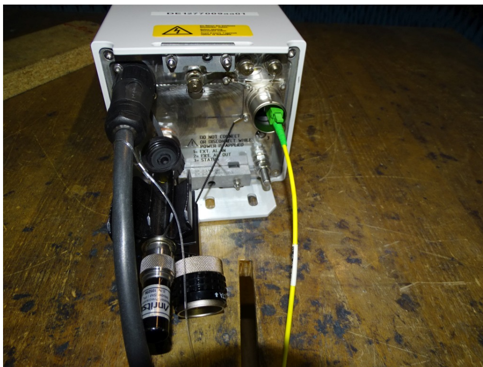
Photo 2: Test setup for radiated emissions measurements in semi-anechoic chamber (30 MHz to 1 GHz), detailed view, termination of RF connectors
