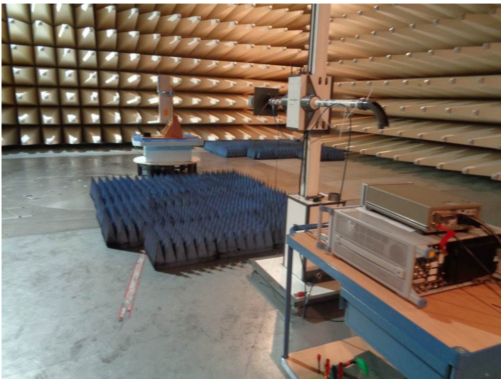
picture 8.4: Test setup: Field Strength Emission 18 – 26.5 GHz @3m in the SAC
