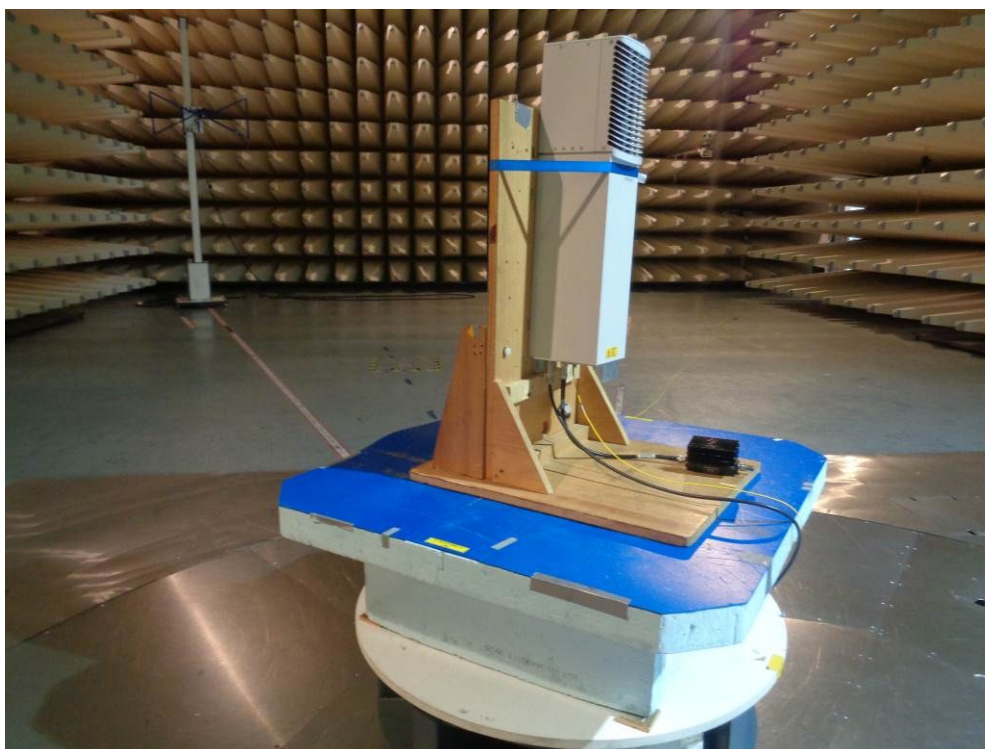
picture 8.2: Test setup: Field Strength Emission 30 M – 1 GHz @10m in the SAC
